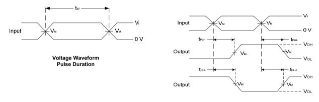
Voltage Waveform Propagation Delay Times
