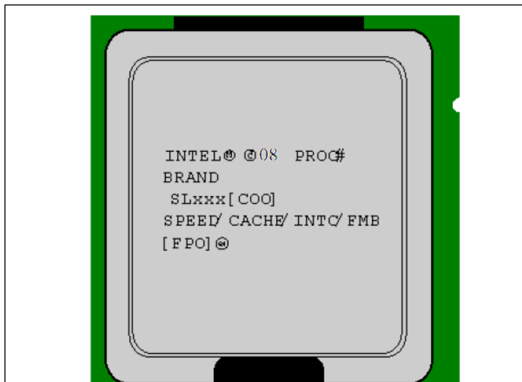
Figure 3-4. Processor Top-Side Markings
