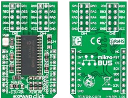
EXPAND Click is an accessory board in **mikroBus™** form factor. It includes a 16-bit I/O expander **MCP23S17** with SPI clock speeds up to 10 MHz for higher throughput applications. Three **HARDWARE ADDRESS SEL** jumpers allow you to configure board address and connect up to eight devices on the bus. Controller also supports interrupt-on-change. Board is set to use 3.3V power supply by default. Solder **PWR SEL** SMD jumper to 5V position if used with 5V systems.
