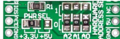
There are four zero-ohm resistors (SMD jumpers): **PWR SEL** is used to determine whether 5V or 3.3V power supply is used, and three **HARDWARE ADDRESS SEL** for selecting the device address.
