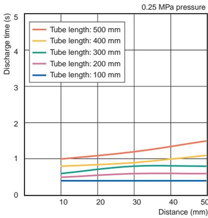
**Standard Nozzle with Conductive Urethane Tube**
