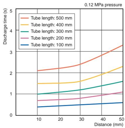
**Standard Nozzle with Fluororesin Tube**
