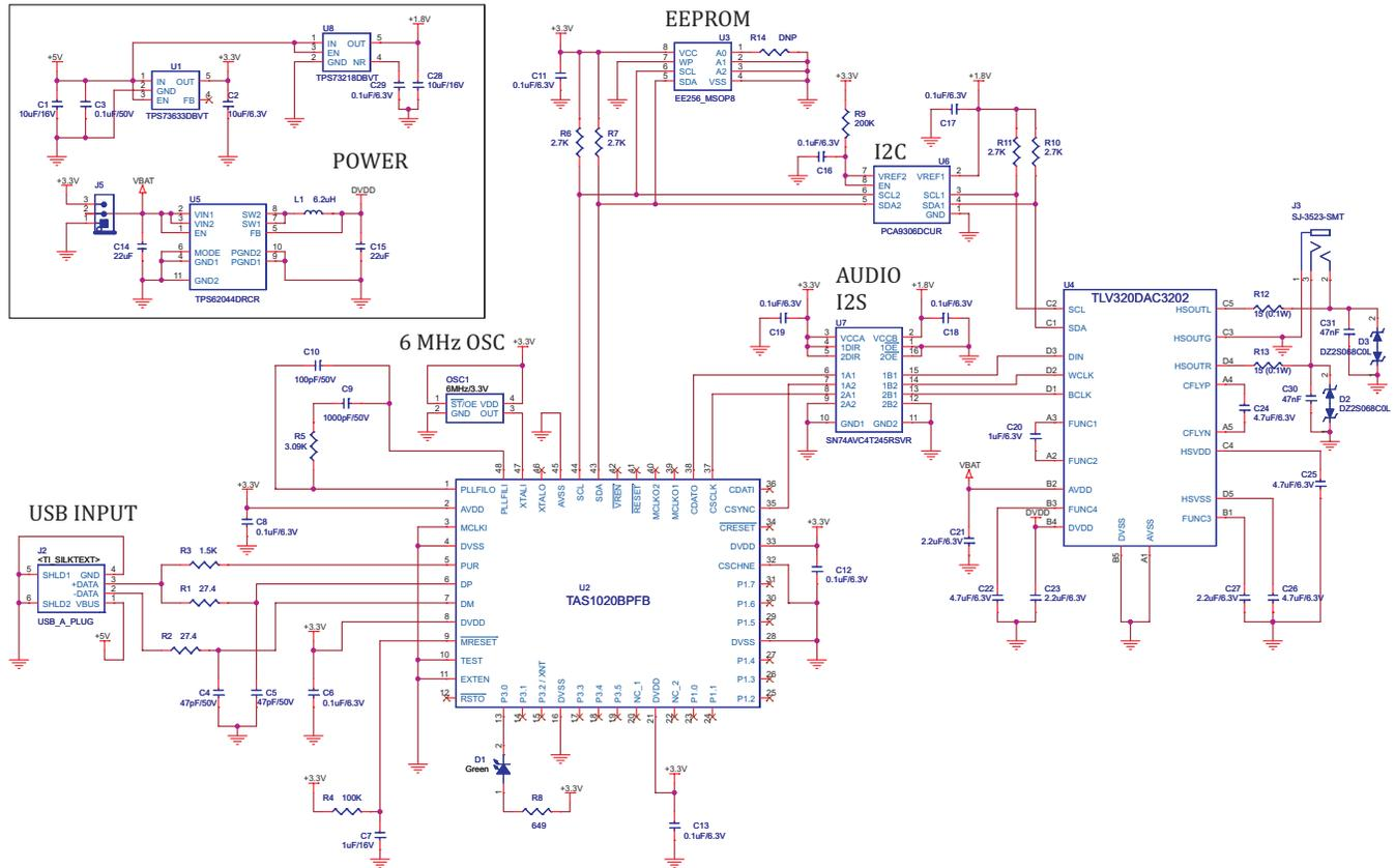
Figure 8. TLV320DAC3202EVM Schematic
