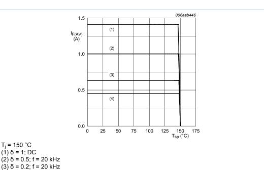
Fig. 12. Average forward current as a function of solder point temperature; typical values
