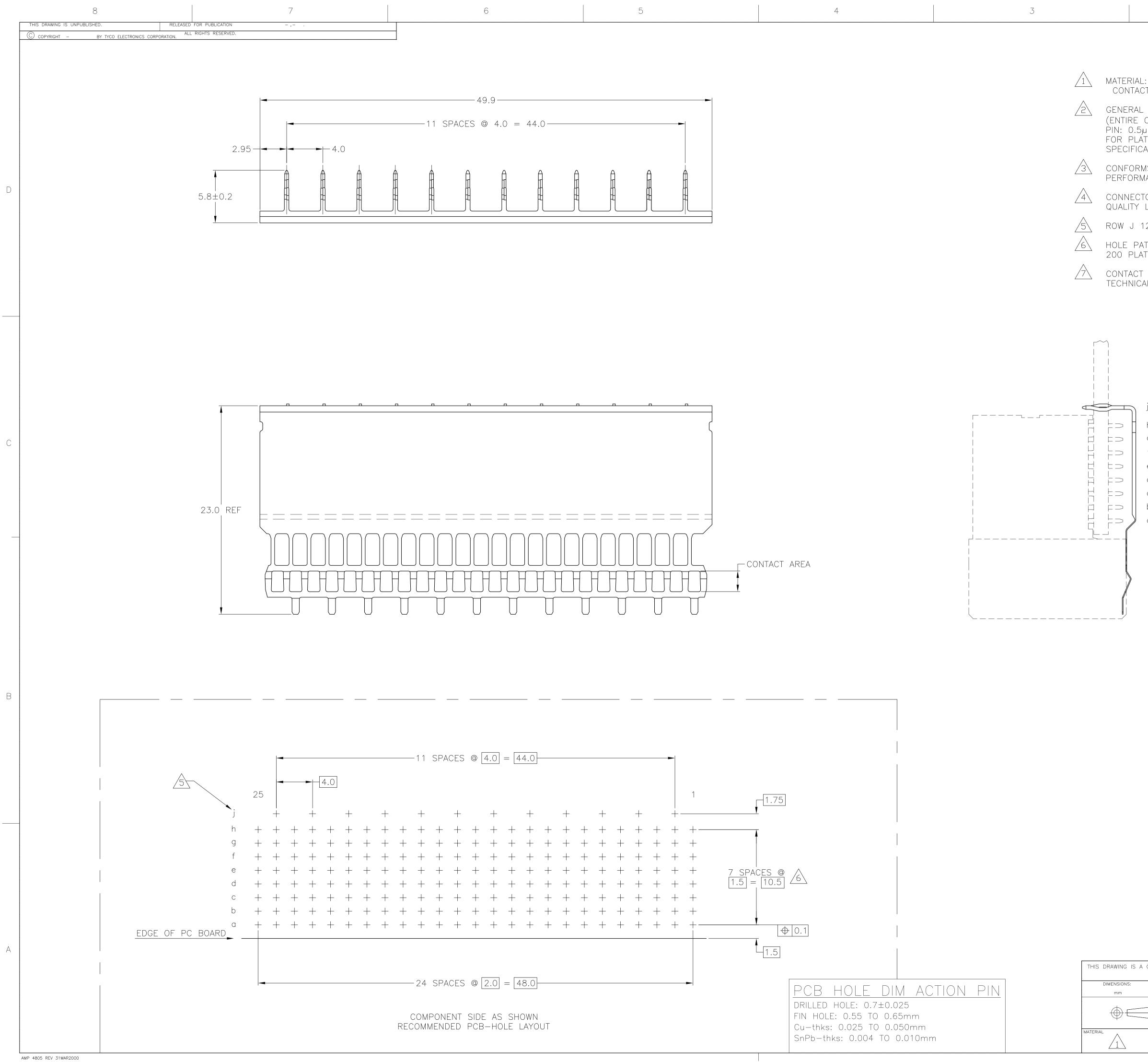
CONTACT AREA LUBRICATED WITH BELLCORE APPROVED LUBRICANT. TECHNICAL REFERENCE: GR-1217-CORE, ISSUE 1, NOVEMBER 1995.
