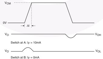
Figure 30. CMR Test Circuit and Waveforms
