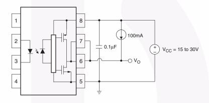
Figure 23. V<sub>OL</sub> Test Circuit
