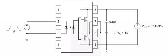
Figure 26. I<sub>FLH</sub> Test Circuit
