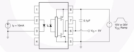
Figure 28. UVLO Test Circuit
