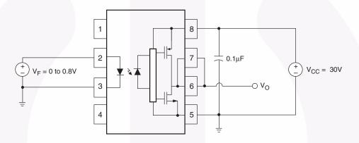
Figure 25. I<sub>CCL</sub> Test Circuit
