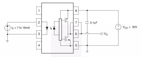
Figure 24. I<sub>CCH</sub> Test Circuit
