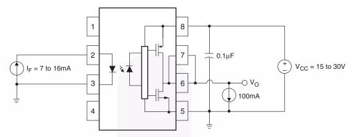
Figure 22. V<sub>OH</sub> Test Circuit
