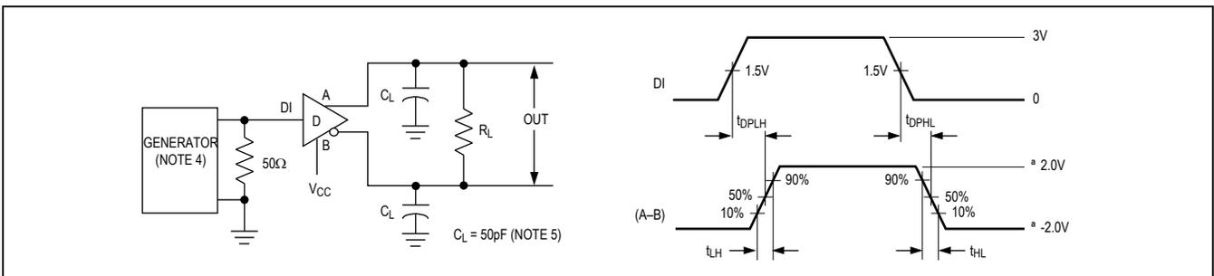
Figure 4. Driver Differential Output Delay and Transition Times
