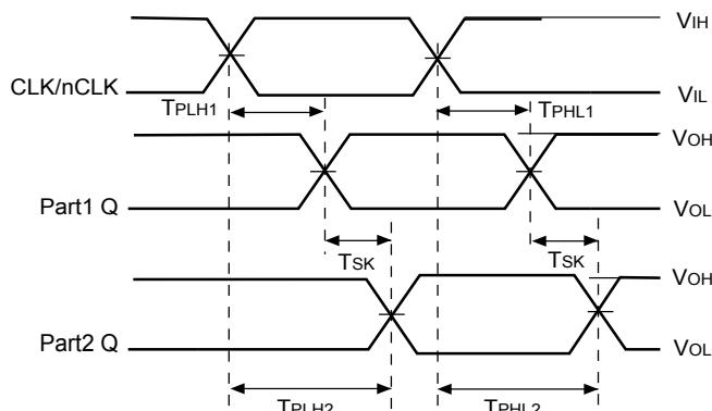
$$T_{SK} = T_{PLH2} - T_{PLH1} \text{ or } T_{SK} = T_{PHL2} - T_{PHL1}$$
