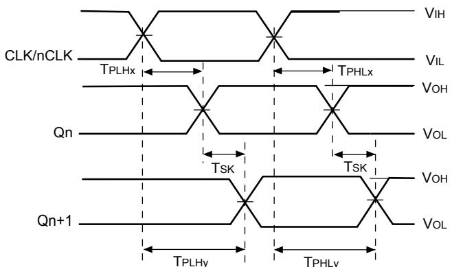
$$T_{SK} = T_{PLHy} - T_{PLHx} \text{ or } T_{SK} = T_{PHLy} - T_{PHLx}$$
