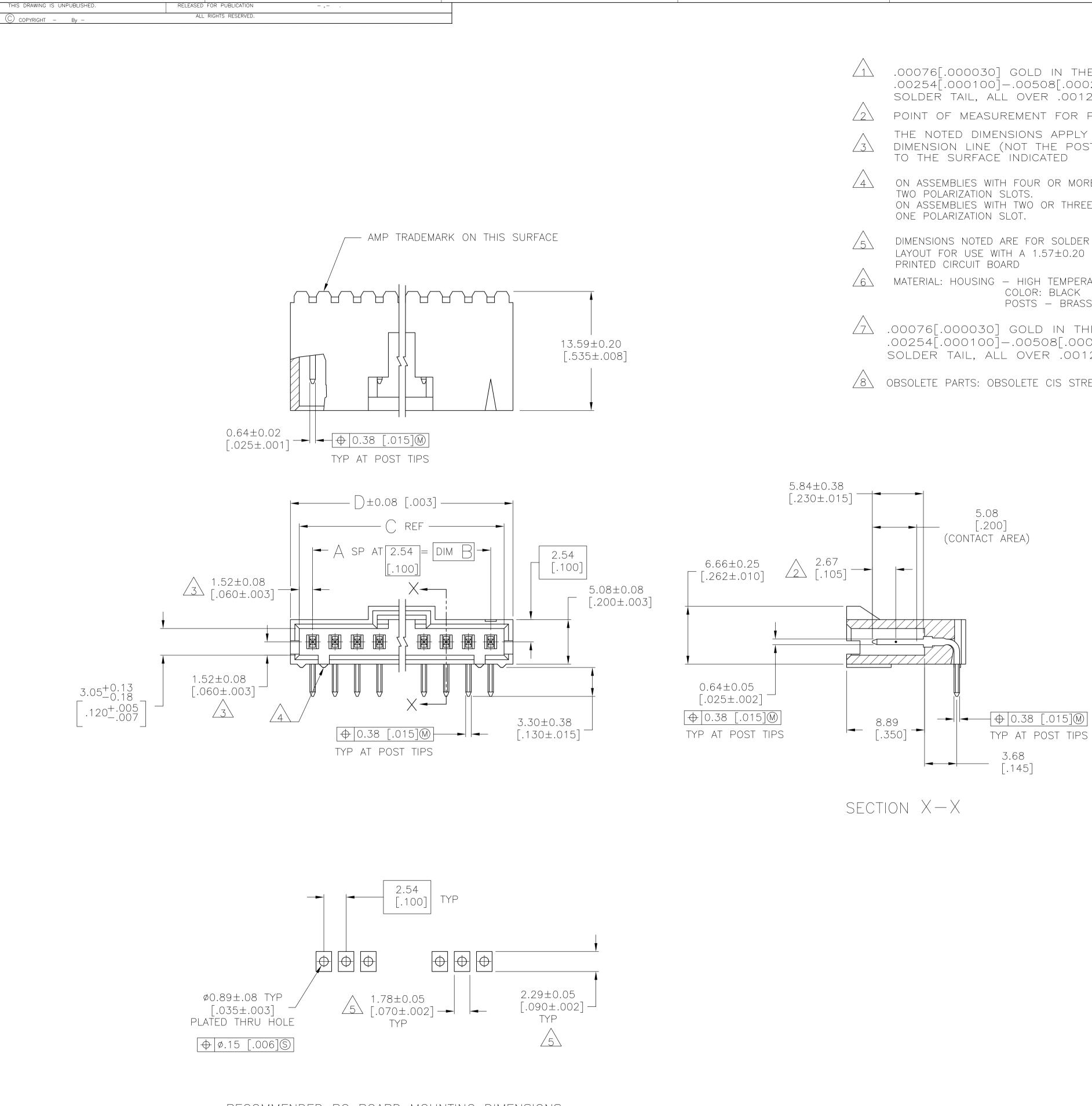
RECOMMENDED PC BOARD MOUNTING DIMENSIONS RECOMMENDED STENCIL THICKNESS = 0.25 [.010]
