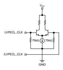
Figure 1. Simplified LVPECL Input Stage
