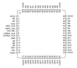
64-Pin EPAD-TQFP (H64-1)
