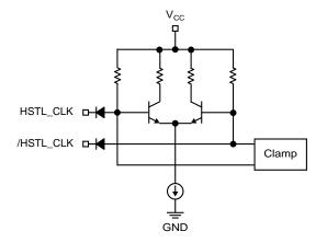
Figure 2. Simplified HSTL Input Stage
