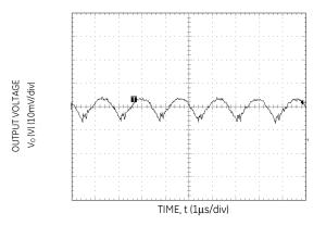
Figure 3. Typical output ripple and noise ( $V_{IN} = 12V$ ,  $I_0 = I_{O,max}$ ).
