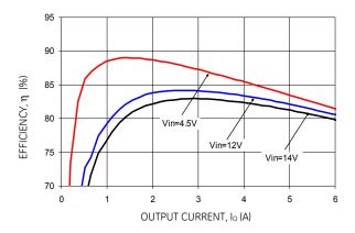
Figure 7. Converter Efficiency versus Output Current.
