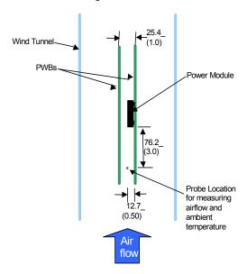
Figure 49. Thermal Test Setup.
