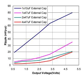
Figure 41. Output ripple voltage for various output voltages with external 1x10  $\mu$ F, 1x47  $\mu$ F, 2x47  $\mu$ F or 4x47  $\mu$ F ceramic capacitors at the output (6A load). Input voltage is 12V.
