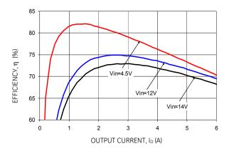
Figure 1. Converter Efficiency versus Output Current.
