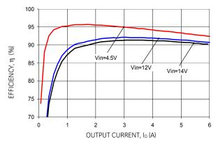
Figure 25. Converter Efficiency versus Output Current.
