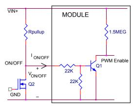
Figure 43. Circuit configuration for using negative On/Off logic.
