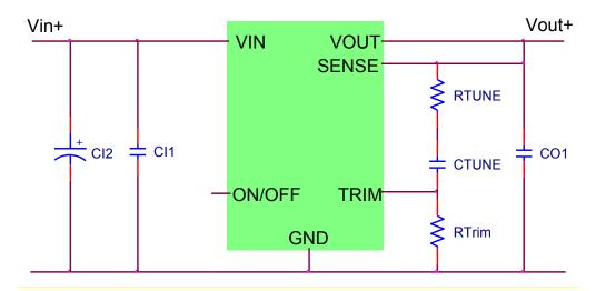
CI1  $22\mu\text{F}/16\text{V}$  ceramic capacitor (e.g. Murata GRM32ER61C226KE20)
