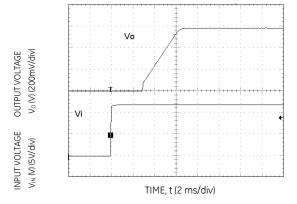
Figure 6. Typical Start-up Using Input Voltage ( $V_{IN} = 12V$ ,  $I_0 = I_{I_0 = 0.01}$ )
