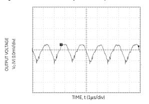
Figure 9. Typical output ripple and noise ( $V_{IN} = 12V$ ,  $I_0 = I_{O,max}$ ).
