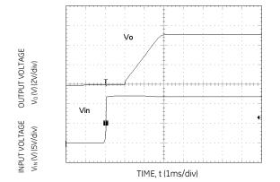
Figure 33. Typical Start-up Using On/Off Voltage ( $I_0 = I_{0,max}$ ).
