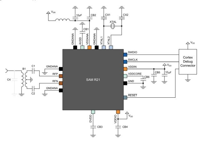
The power supply decoupling capacitors (CB2, CB4, CB5) are connected to the external analog supply VDDANA, the external digital supplies VDDIO and VDDIN. Capacitors CB1, CB3 and CB6 are bypass capacitors for the integrated analog and digital voltage regulators to ensure stable operation. All bypass capacitors should be placed as close as possible to the pins and should have a low-resistance and low-inductance connection to ground to achieve the best performance.
