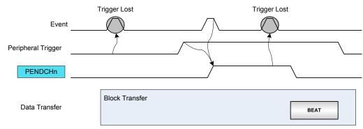
**Conditional transfer:** When the conditional transfer event action is selected, the event input is used to trigger a conditional transfer on peripherals with pending transfer requests. As example, this type of event can be used for peripheral to peripheral transfers, where one peripheral is source of event and the second peripheral is source of DMA trigger.
