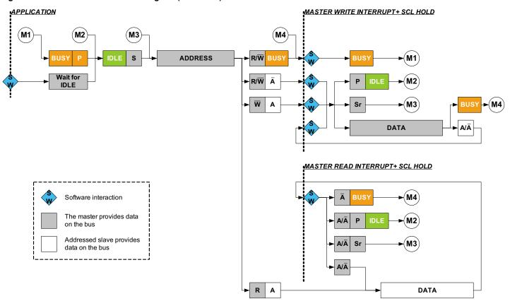
In the second strategy (SCLSM=1), interrupts only occur after the ACK bit as shown in Figure 26-7. This strategy can be used when it is not necessary to check DATA before acknowledging.
