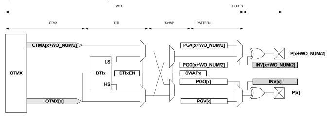
The output matrix (OTMX) unit distributes compare channels, according to the selectable configurations, as shown in Table 28-3.
