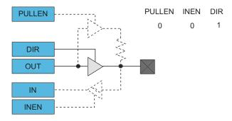
Figure 21-7. I/O Configuration - Totem-Pole Output with Enabled Input
