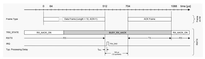
Note: If register bit AACK\_ACK\_TIME (register 0x17, XAH\_CTRL\_1) is set, an acknowledgment frame is sent already two symbol times after the reception of the last symbol of a data or MAC command frame.
