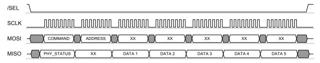
Figure 35-14.Example SPI Sequence - SRAM Write Access of a 5-byte Data Package
