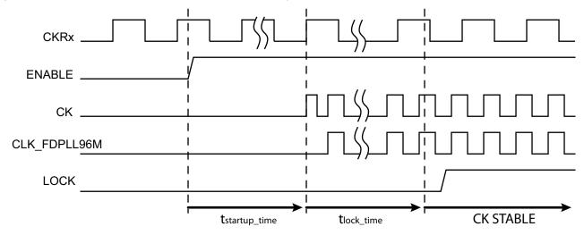
Figure 15-5. CK and CLK\_FDPLL96M Running Mode to Off Mode
