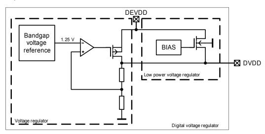
The block "Low power voltage regulator" within the "Digital voltage regulator" maintains the DVDD supply voltage at 1.5V (typical) when the AT86RF233 voltage regulator is disabled in sleep mode. All configuration register values are stored.
