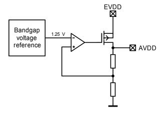
A simplified schematic of the internal digital voltage regulator is shown in Figure 38-6.
