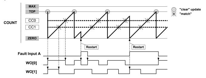
Figure 28-27. Waveform Generation in RAMP2 Mode with Restart Action
