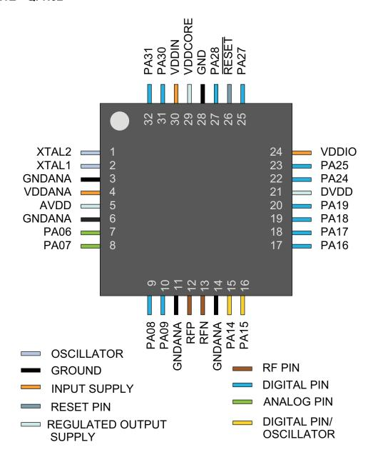
Note: The large center pad underneath the QFN package is made of metal and internally connected to GND. It should be soldered and connected to the digital ground on the board to ensure good mechanical stability. It is not recommended to use the exposed paddle as a replacement of the regular GND pin.
