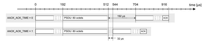
If register bit AACK\_ACK\_TIME (register 0x17, XAH\_CTRL\_1) is set the acknowledgment time is reduced from 192μs to 32μs.
