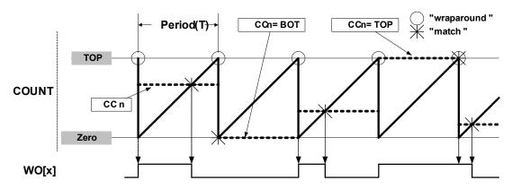
In match operation, Compare/Capture register CC0 is used as the top value, in this case a negative pulse will appear on WO[0] on every overflow/underflow.
