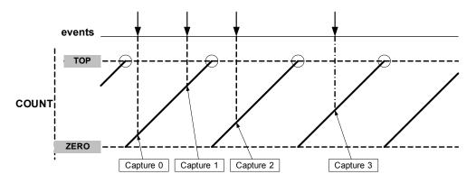
When the Capture Interrupt flag is set and a new capture event is detected, there is nowhere to store the new timestamp. As a result, the Error Interrupt flag in the Interrupt Flag Status and Clear register (INTFLAG.ERR) is set.
