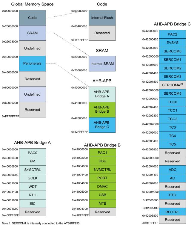
This figure represents the full configuration of the Atmel | SMART SAM R21 with maximum Flash and SRAM capabilities and a full set of peripherals. Refer to the "Configuration Summary" on page 4 for details.
