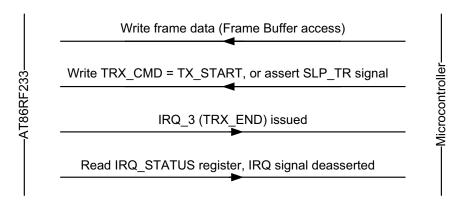
Alternatively for time critical applications when the frame start transmission time needs to be minimized, a frame transmission task can be started first. Then it can be followed by the Frame Buffer write access event (populating PSDU data). This way the data to be transmitted is needs to be written in the transmit frame buffer as the transceiver initializes and begins SHR transmission; refer to Figure 39-3.
