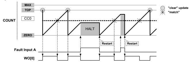
Figure 28-31. Waveform Generation with Fault Qualification, Halt and Restart Actions
