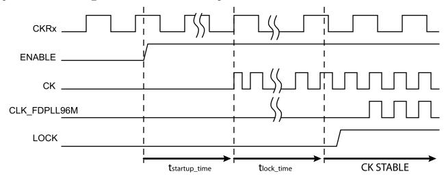
Figure 15-4. CK and CLK\_FDPLL96M Off Mode to Running Mode when Wake-Up Fast is Activated
