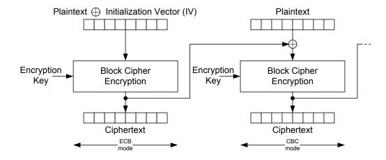
After preparing the AES key and defining the AES operation direction using Atmel AT86RF233 SRAM register bit AES\_DIR, the data has to be provided to the AES engine and the CBC operation can be started.
