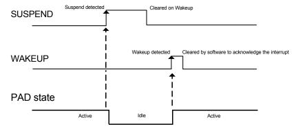
The Suspend Interrupt bit in the Device Interrupt Flag register (INTFLAG.SUSPEND) is set when a USB Suspend state has been detected on the USB bus. The USB pad is then automatically put in the Idle state. The detection of a non-idle state sets the Wake Up Interrupt bit in INTFLAG(INTFLAG.WAKEUP) and wakes the USB pad.
