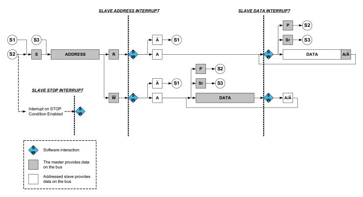
In the second strategy (SCLSM=1), interrupts only occur after the ACK bit as shown in Figure 26-11. This strategy can be used when it is not necessary to check DATA before acknowledging. For master reads, an address and data interrupt will be issued simultaneously after the address acknowledge, while for master writes, the first data interrupt will be seen after the first data byte has been received by the slave and the acknowledge bit has been sent to the master.
