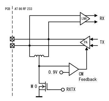
The RF port DC values depend on the operating state; refer to "AT86RF233 Operating Modes" on page 902. In TRX\_OFF state, when the analog front-end is disabled (see "TRX\_OFF – Clock State" on page 904), the RF pins are pulled to ground, preventing a floating voltage larger than 1.8V which is not allowed for the internal circuitry.
