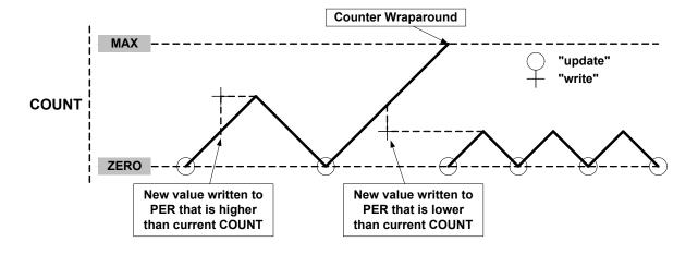
When double buffering is used, the buffer can be written at any time and the counter will still maintain correct operation. The period register is always updated on the update condition, as shown for dual-slope operation in Figure 28-15. This prevents wraparound and the generation of odd waveforms.
