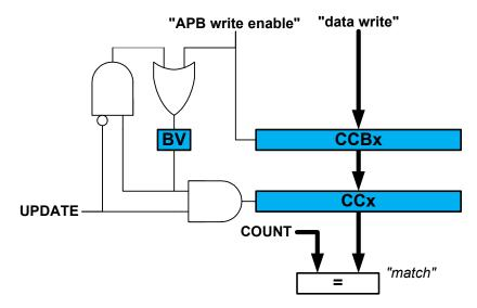
As both the register (PATT/WAVE/PER/CCx) and corresponding buffer register (PATTB/WAVEB/PERB/CCBx) are available in the I/O register map, the double buffering feature is not mandatory. The double buffering is disabled by writing a one to CTRLSET.LUPD. This allows initialization and bypassing of the buffer register and the double buffering feature.
