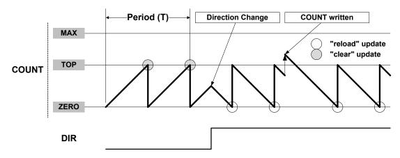
As shown in Figure 28-5, it is possible to change the counter value (by writing directly in the Count register) even when the counter is running. The write access has higher priority than count, clear, or reload. The direction of the counter can also be changed during normal operation. Due to asynchronous clock domains, the internal counter settings are written when the synchronization is complete.
