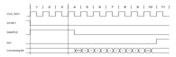
Figure 30-5. ADC Timing for Free Running in Differential Mode without Gain
