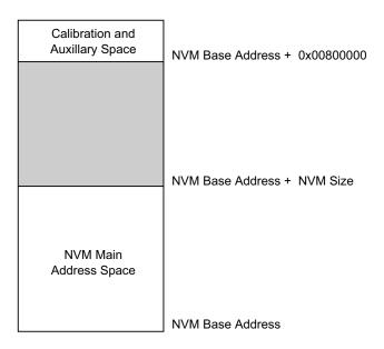
The lower rows in the NVM main address space can be allocated as a boot loader section by using the BOOTPROT fuses, and the upper rows can be allocated to EEPROM emulation, as shown in Figure 20-4. The boot loader section is protected by the lock bit(s) corresponding to this address space and by the BOOTPROT[2:0] fuse. The EEPROM rows
