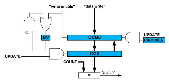
Figure 28-19. Circular Buffer on Channel 0
