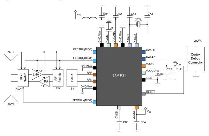
In this example, a balun (B1) transforms the differential RF signal at the SAM R21 radio transceiver RF pins (RFP/RFN) to a single ended RF signal, similar to the Basic Application Schematic; refer to Figure 34-1. During receive mode the radio transceiver searches for the most reliable RF signal path using the Antenna Diversity algorithm. One antenna is selected (SW2) by the Antenna Diversity RF switch control signal (DIG1), refer to "Antenna Diversity" on page 1020.
