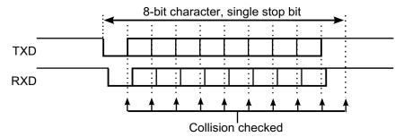
Figure 24-12 shows the conditions for a collision detection. In this case, the start bit and the first data bit are received with the same value as transmitted. The second received data bit is found to be different than the transmitted bit at the detection point which indicates a collision.
