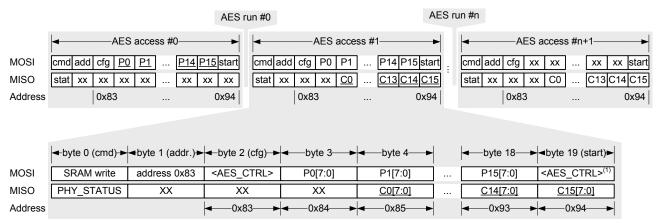
Note: 1. Byte 19 is the mirrored version of register AES\_CTRL on SRAM address 0x94, see register description AES\_CTRL\_MIRROR for details.
