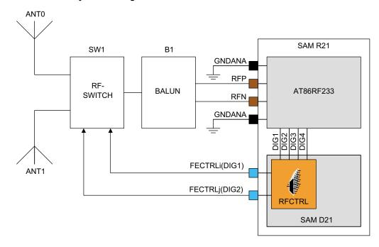
Generally, when the external RF-Switch (SW1) is to be controlled by antenna diversity algorithm, the antenna diversity enable must be activated by register bit ANT\_EXT\_SW\_EN (register 0x0D, ANT\_DIV). Then the internal digital control signals DIG1 and DIG2 are enabled (refer to "Digital I/O Signals" on page 18) to drive the antenna switch control signals to the differential inputs of the RF Switch (SW1) to switch between ANT0 and ANT1.
