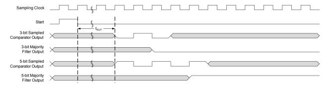
During sleep modes, filtering is supported only for single-shot measurements. Filtering must be disabled if continuous measurements will be done during sleep modes, or the resulting interrupt/event may be generated incorrectly.
