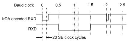
Note that the polarity of the transmitter and receiver are opposite. During transmission, a zero bit is transmitted as a one pulse. During reception, an accepted zero pulse is received as a zero bit.
