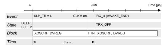
The AT86RF233 radio transceiver's DEEP\_SLEEP state is left by releasing SLP\_TR to logic low. This restarts the XOSCRF and DVREG. After  $t_{TR18}$  = 360 $\mu$ s (typ.) the radio transceiver enters TRX\_OFF state. The internal clock signal is available and provided at a default rate of 1MHz to CLKM.
