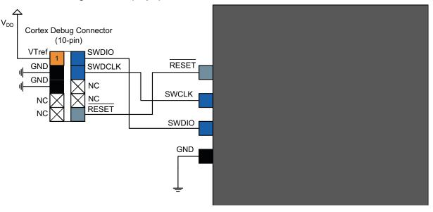
Table 45-9. Cortex Debug Connector (10-pin)
