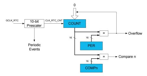
Figure 17-3. RTC Block Diagram (Mode 2 — Clock/Calendar)
