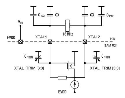
Additional internal trimming capacitors  $C_{TRIM}$  are available. Any value in the range from 0pF to 4.5pF with a 0.3pF resolution is selectable using XTAL\_TRIM of register 0x12 (XOSC\_CTRL). To calculate the total load capacitance, the following formula can be used:
