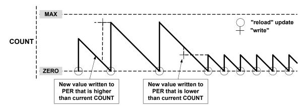
A counter wraparound can occur in any mode of operation when up-counting without buffering, as shown in Figure 28-12. This due to the fact that COUNT and TOP are continuously compared, and if a new value that is lower than the current COUNT is written to TOP, COUNT will wrap before a compare match happen.
