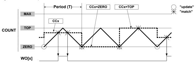
Using dual-slope PWM results in a lower maximum operation frequency compared to single-slope PWM generation.
