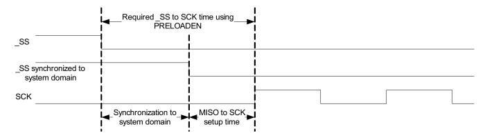
Only one data character written to DATA will be preloaded into the shift register while the synchronized \_SS signal (see Figure 25-4) is high. The next character written to DATA before \_SS is pulled low will be stored in DATA until transfer begins. If the shift register is not preloaded, the current contents of the shift register will be shifted out.
