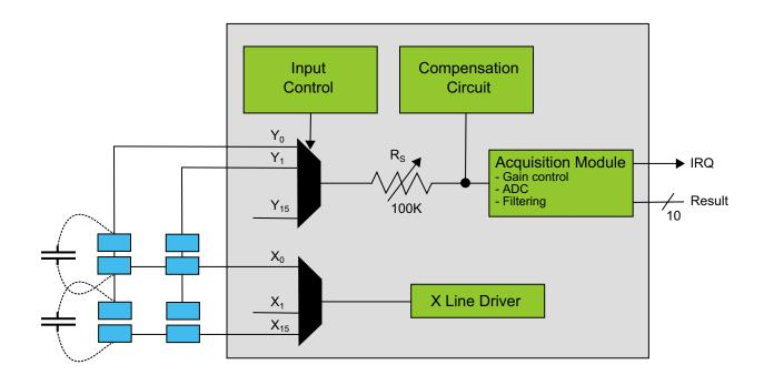
Figure 32-2. PTC Block Diagram Self-capacitance
