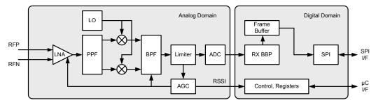
The differential RF signal is amplified by a low noise amplifier (LNA), filtered (PPF) and down converted to an intermediate frequency by a mixer. Channel selectivity is performed using an integrated band pass filter (BPF). A limiting amplifier (Limiter) provides sufficient gain to overcome the DC offset of the succeeding analog-to-digital converter (ADC) and generates a digital RSSI signal. The ADC output signal is sampled and processed further by the digital base band receiver (RX BBP).
