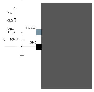
A pull-up resistor makes sure that the reset does not go low unintended causing a device reset. An additional resistor has been added in series with the switch to safely discharge the filtering capacitor, i.e. preventing a current surge when shorting the filtering capacitor which again causes a noise spike that can have a negative effect on the system.
