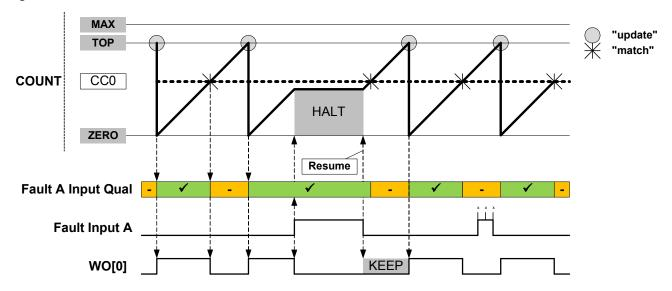
The software halt action can be configured using Faultn Halt mode bits in Recoverable Faultn configuration register (FCTRLn.HALT = SWHALT). Software halt action is similar to hardware halt action with one exception. To restart the timer/counter, the corresponding fault condition should no longer be present and the corresponding FAULTn bit in STATUS register must be cleared.
