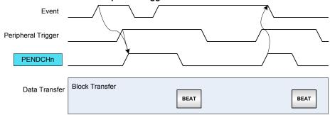
**Conditional block transfer:** When the conditional block event action is selected, the event input is used to trigger a conditional block transfer on peripherals. The peripheral Trigger Source must be set in Channel Control B register (CHCTRLB.TRIGSRC).
