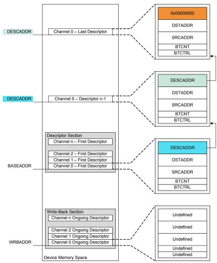
The size of the descriptor and write-back memory sections is dependant on most significant enabled DMA channel, as shown below:
