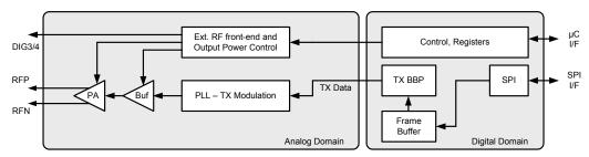
The TX BBP reads the frame data from the Frame Buffer and performs the bit-to-symbol and symbol-to-chip mapping as specified by IEEE 802.15.4 in Section 6.5.2. The O-QPSK modulation signal is generated and fed into the analog radio front end.
