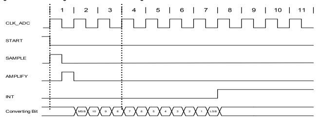
Figure 30-7. ADC Timing for Free Running in Single-Ended Mode without Gain
