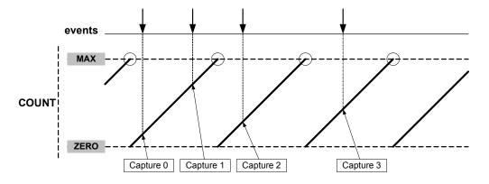
For input capture, the buffer register and the corresponding CCx act like a FIFO. When CCx is empty or read, any content in CCBx is transfered to CCx. The buffer valid flag is passed to set the CCx interrupt flag (IF) and generate the optional interrupt, event or DMA request.
