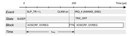
The radio transceiver's SLEEP state is left by releasing SLP\_TR to logic low. This restarts the XOSCRF and DVREG. After  $t_{TR2}$  = 210 $\mu$ s (typ.) the radio transceiver enters TRX\_OFF state. The internal clock signal is available and provided by CLKM, if enabled.
