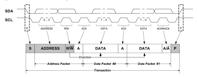
Figure 26-3. Transaction Diagram Syntax
