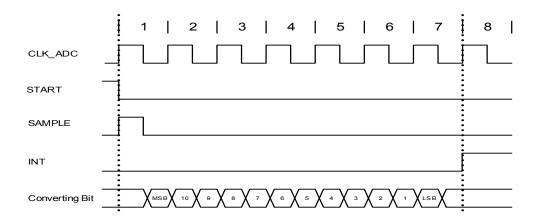
Figure 30-4. ADC Timing for One Conversion in Differential Mode without Gain, but with Increased Sampling Time
