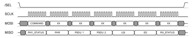
Figure 35-10. Example SPI Sequence - Frame Buffer Write of a Frame with 4-byte PSDU
