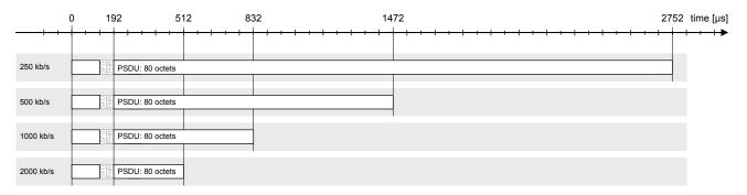
Due to the overhead caused by the SHR, PHR as well as the FCS, the effective data rate is lower than the selected data rate. This is also affected by the length of the PSDU. A graphical representation of the effective PSDU data rate is shown in Figure 40-7.
