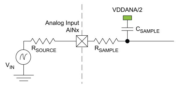
To achieve n bits of accuracy, the  $C_{SAMPLE}$  capacitor must be charged at least to a voltage of  $V_{CSAMPLE} \ge V_{IN} \times (1-2^{-(n+1)})$
