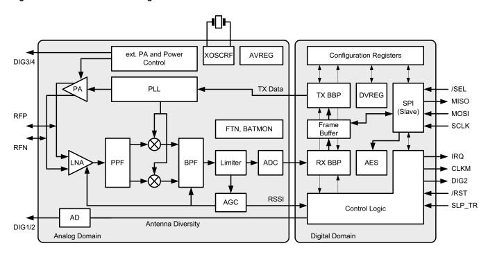
The number of external components is minimized such that only the antenna, the crystal and decoupling capacitors are required. The bidirectional differential antenna pins (RFP, RFN) are used for transmission and reception, thus no external antenna switch is needed. Control of an external power amplifier is supported by two digital control signals (differential operation).
