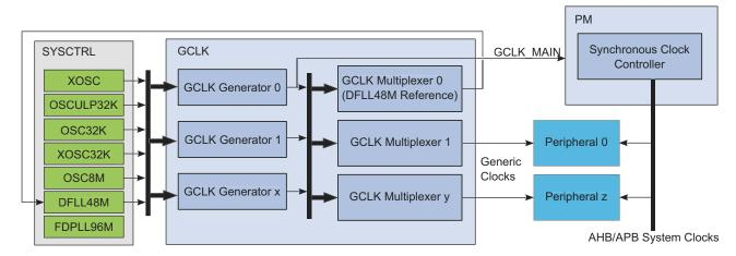
The clock system on the SAM R21 consists of:
