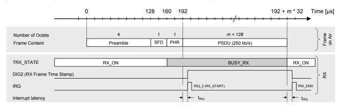
Note: 1. Timing figures  $t_{IRQ}$  refer to "Digital Interface Timing Characteristics" on page 1101.
