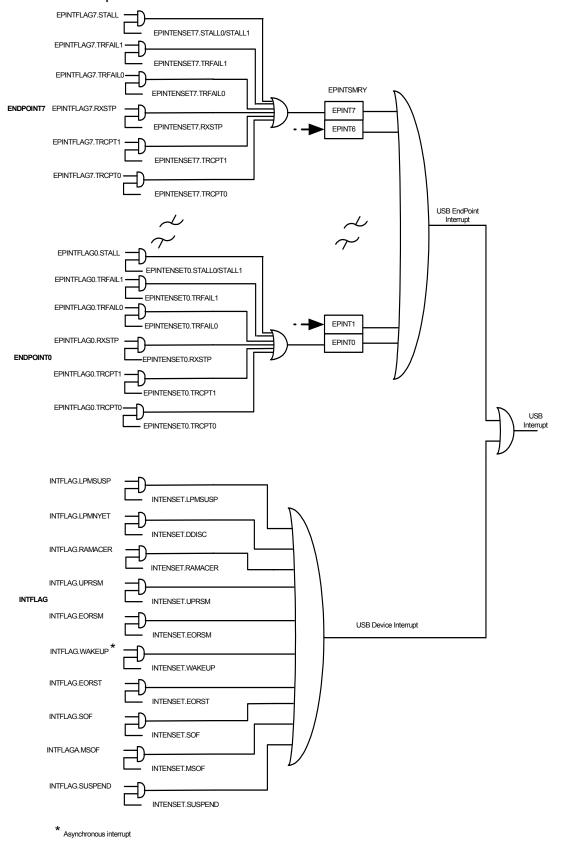
The WAKEUP is an asynchronous interrupt and can be used to wake-up the device from any sleep mode.
