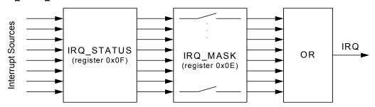
The AT86RF233 IRQ signal polarity can be configured with register bit IRQ\_POLARITY (register 0x04, TRX\_CTRL\_1). The default behavior is active high, which means that the signal IRQ = H issues an interrupt request.
