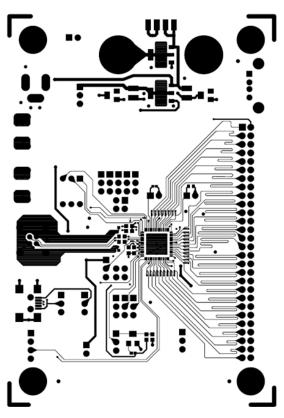
Figure 45. DS90UR906Q-Q1 Deserializer Example Layout
