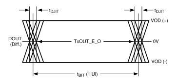
Figure 8. Serializer Output Jitter
