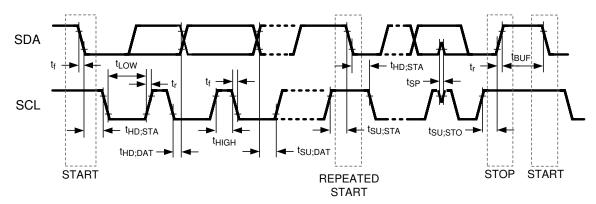
Figure 18. Serial Control Bus Timing Diagram
