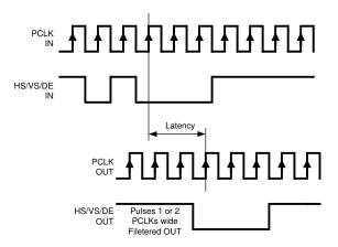
Figure 24. Video Control Signal Filter Waveform
