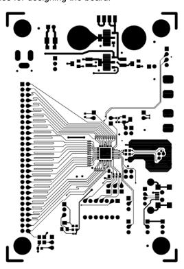
Figure 44. DS90UR905Q-Q1 Serializer Example Layout
