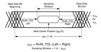
Figure 16. Receiver Input Jitter Tolerance
