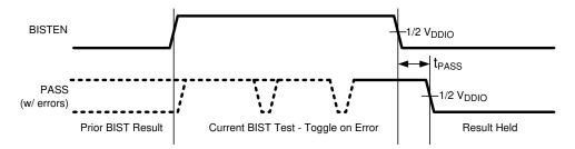
Figure 17. BIST PASS Waveform
