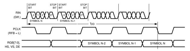
Figure 11. Deserializer Delay – Latency
