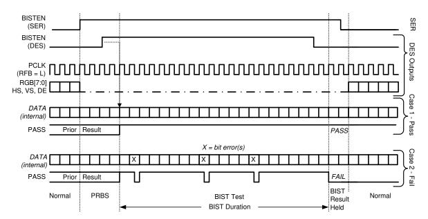
Figure 33. BIST Waveforms
