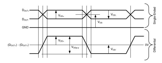
Figure 2. Serializer Output Waveforms
