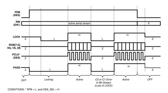
Figure 28. Deserializer Outputs With Output State Select High (OSS\_SEL = H)
