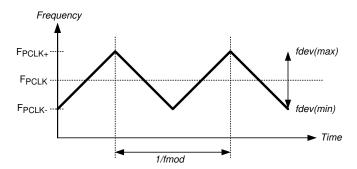
Figure 26. SSCG Waveform
