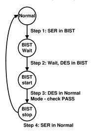
Figure 32. BIST Mode Flow Diagram
