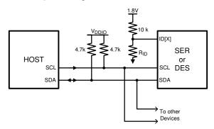
Figure 34. Serial Control Bus Connection
