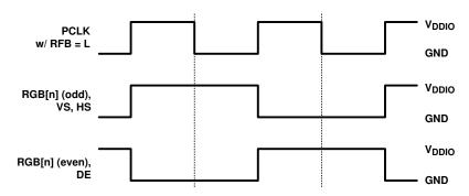
Figure 9. Checkerboard Data Pattern
