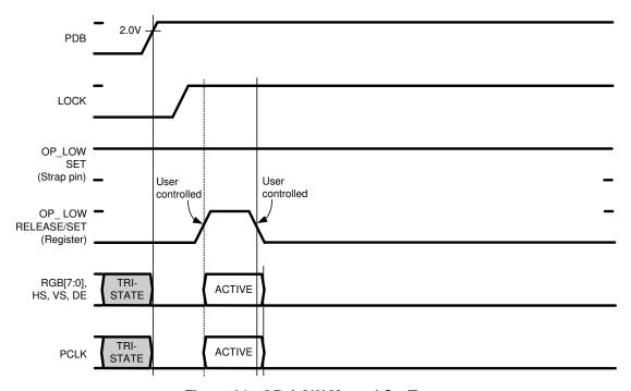
Figure 31. OP\_LOW Manual Set/Reset
