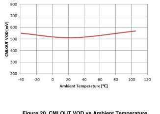
Figure 20. CMLOUT VOD vs Ambient Temperature
