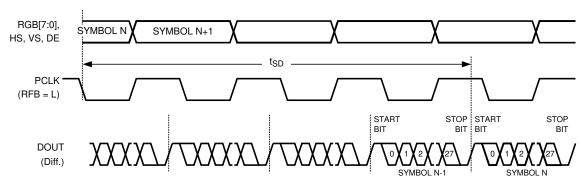
Figure 7. Serializer Latency Delay
