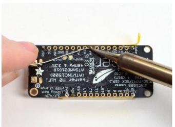
Be sure to solder all pins for reliable electrical contact.
