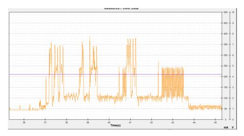
Sending an MQTT packet (about 200 bytes)
