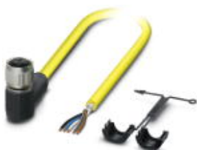
Sensor/actuator cable, 5-position, PVC, yellow, shielded, free cable end, on Socket angled M12 SPEEDCON, A-coded, cable length: 5 m
