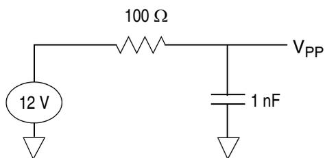
**Figure 35. Example V<sub>PP</sub> Filtering**
