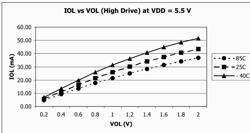
Figure 24. Typical  $I_{OL}$  vs.  $V_{OL}$
