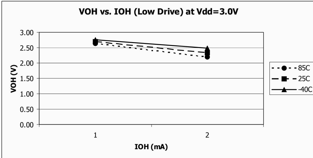
Figure 9. Typical  $V_{OH}$  vs.  $I_{OH}$
