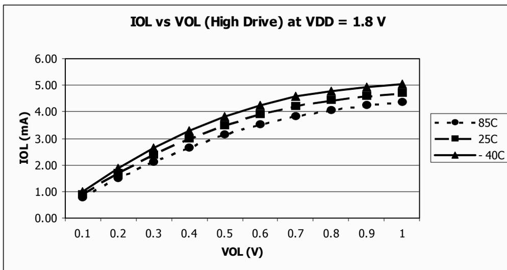
Figure 28. Typical  $I_{OL}$  vs.  $V_{OL}$
