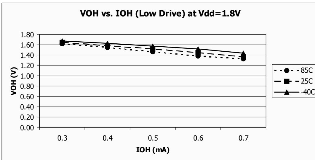
Figure 11. Typical  $V_{OH}$  vs.  $I_{OH}$
