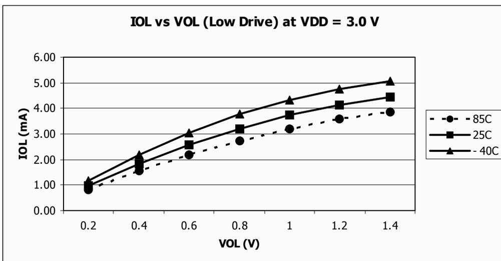
Figure 27. Typical  $I_{OL}$  vs.  $V_{OL}$
