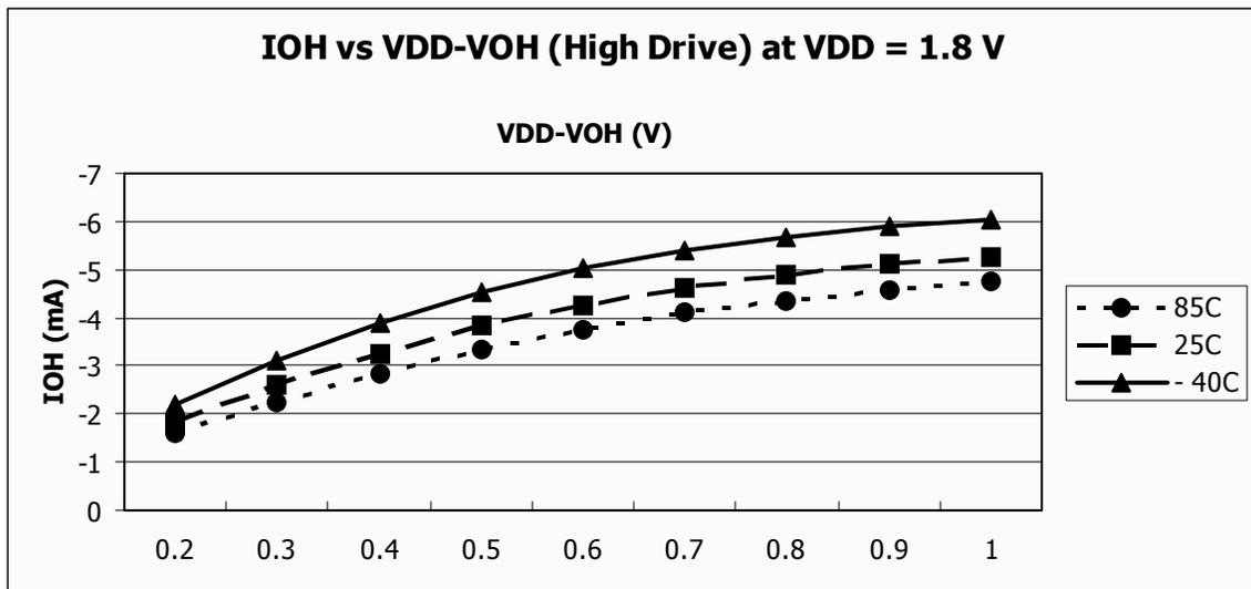
Figure 22. Typical  $I_{OH}$  vs.  $V_{DD}-V_{OH}$
