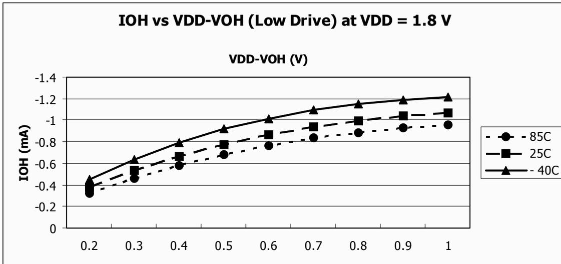
Figure 23. Typical  $I_{OH}$  vs.  $V_{DD}-V_{OH}$
