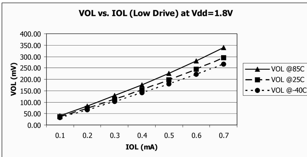
Figure 17. Typical  $V_{OL}$  vs.  $I_{OL}$
