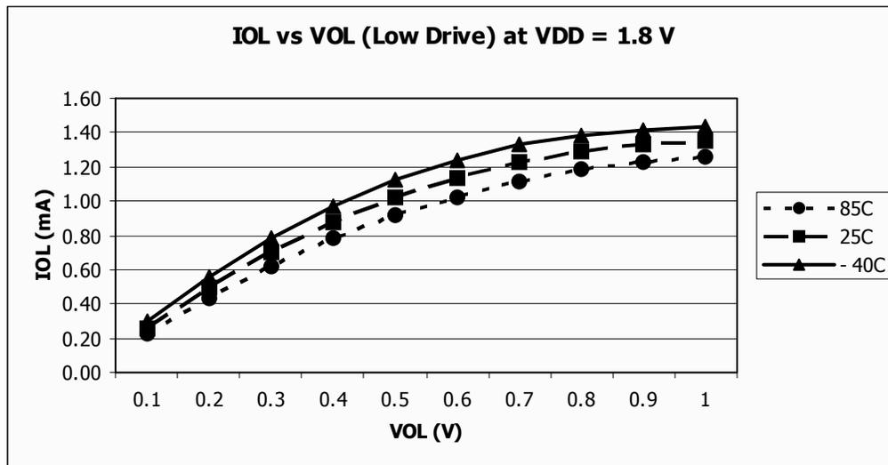
Figure 29. Typical  $I_{OL}$  vs.  $V_{OL}$
