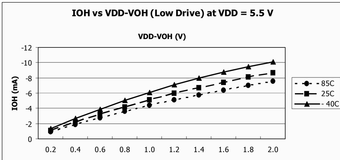
Figure 19. Typical I<sub>OH</sub> vs. V<sub>DD</sub>-V<sub>OH</sub>
