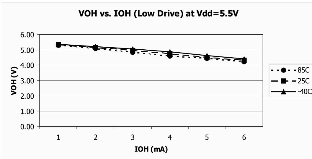
Figure 7. Typical  $V_{OH}$  vs.  $I_{OH}$
