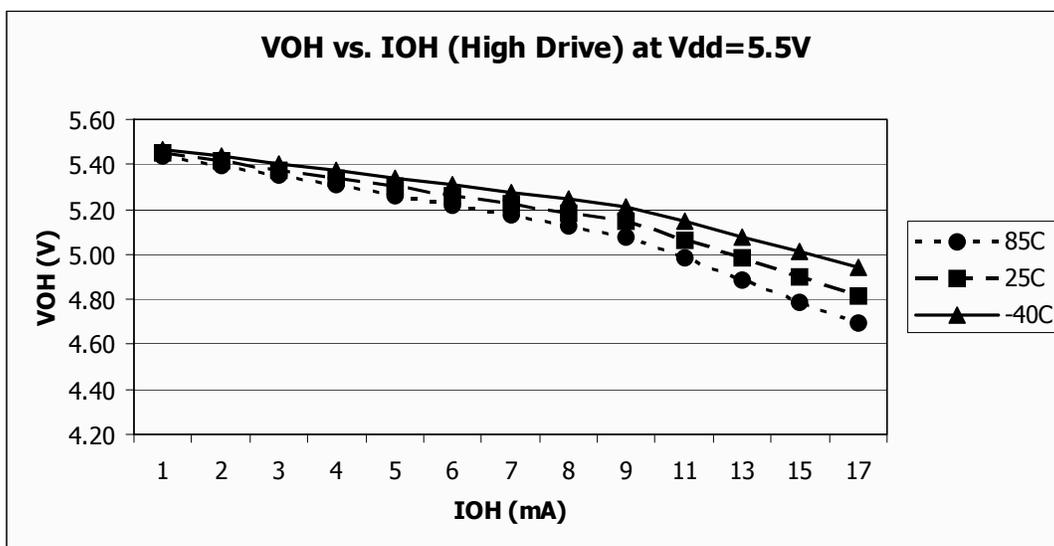
Figure 18. Typical  $I_{OH}$  vs.  $V_{DD}-V_{OH}$
