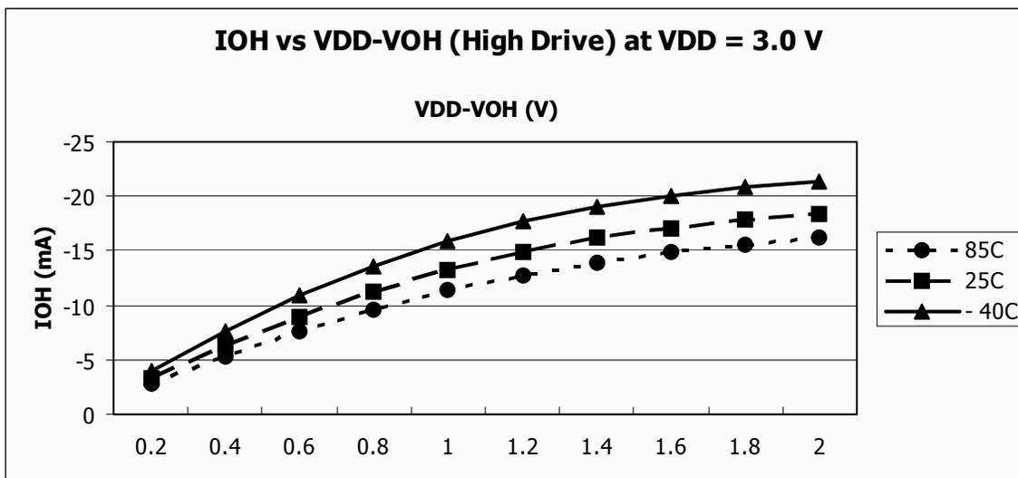
Figure 20. Typical I<sub>OH</sub> vs. V<sub>DD</sub>-V<sub>OH</sub>
