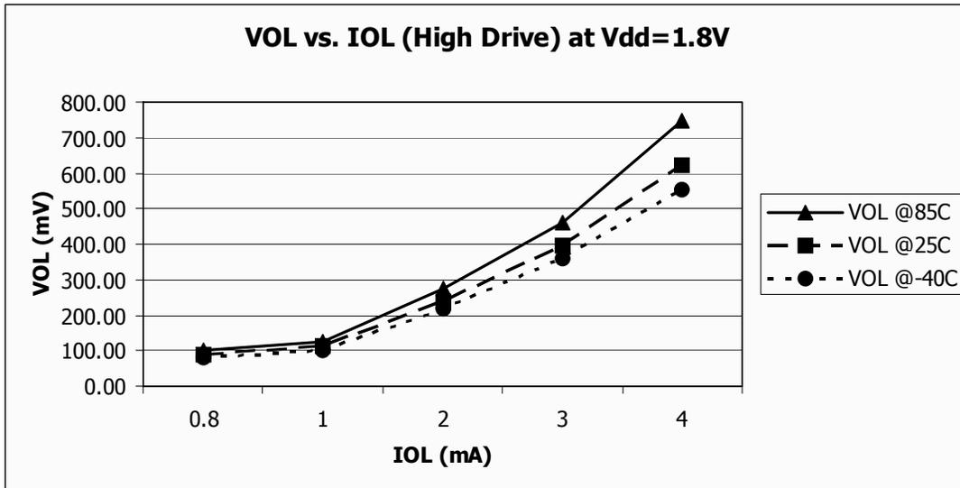
Figure 16. Typical  $V_{OL}$  vs.  $I_{OL}$
