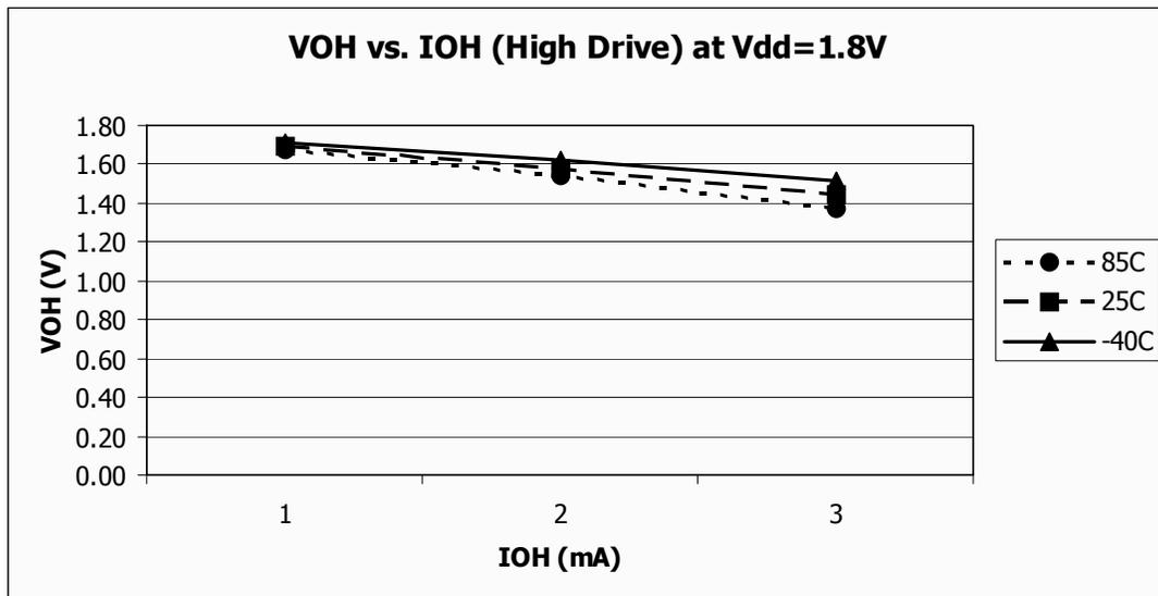
Figure 10. Typical  $V_{OH}$  vs.  $I_{OH}$
