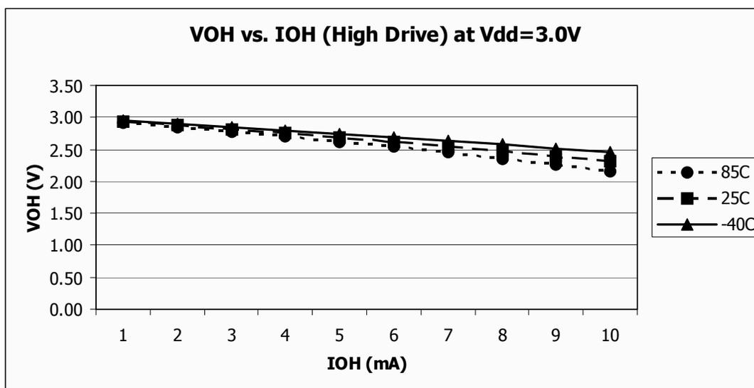
Figure 8. Typical  $V_{OH}$  vs.  $I_{OH}$
