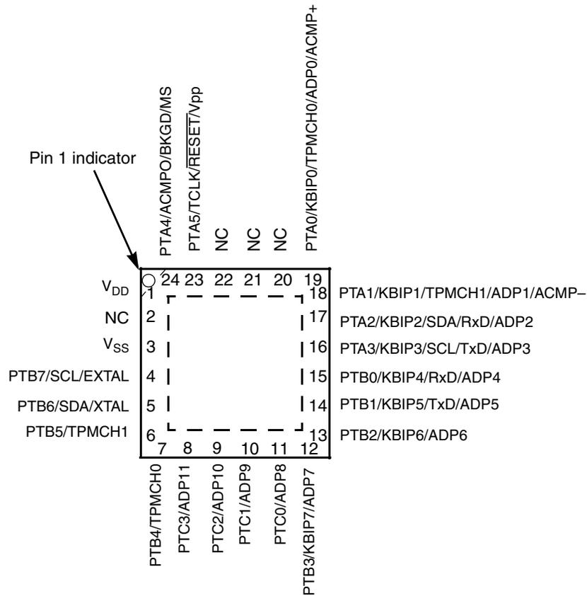
Figure 2. MC9RS08KB12 Series 24-Pin QFN Package
