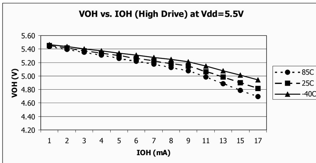
**Figure 6. Typical  $V_{OH}$  vs.  $I_{OH}$
