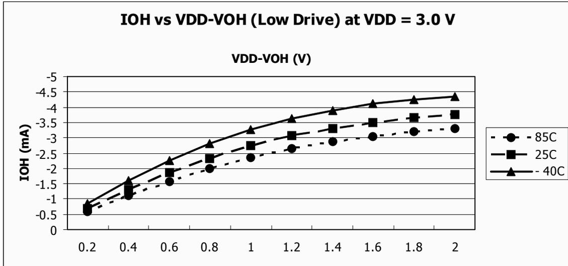
Figure 21. Typical  $I_{OH}$  vs.  $V_{DD}-V_{OH}$
