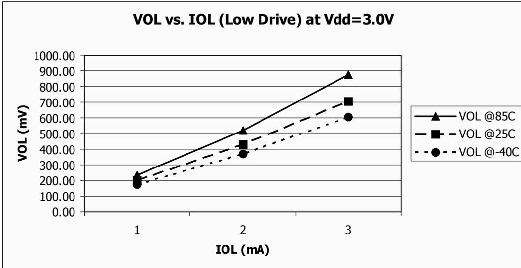
Figure 15. Typical  $V_{OL}$  vs.  $I_{OL}$
