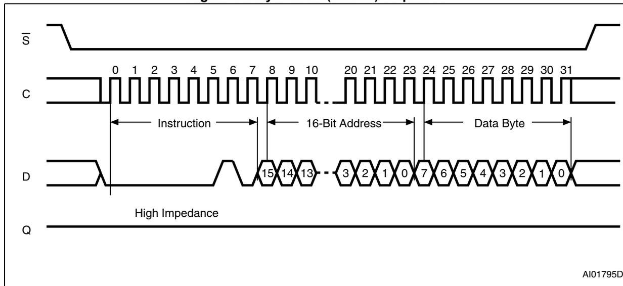
1. Depending on the memory size, as shown in [Table 4](#), the most significant address bits are Don't Care.
