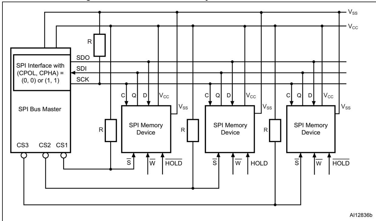
1. The Write Protect ( $\bar{W}$ ) and Hold ( $\overline{HOLD}$ ) signals should be driven, high or low as appropriate.
