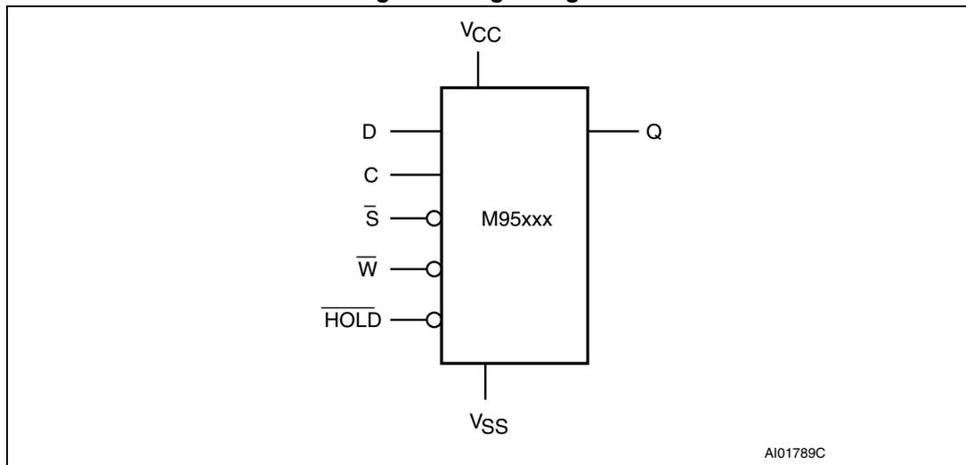
The SPI bus signals are C, D and Q, as shown in [Figure 1](#) and [Table 1](#). The device is selected when Chip Select ( $\bar{S}$ ) is driven low. Communications with the device can be interrupted when the HOLD is driven low.
