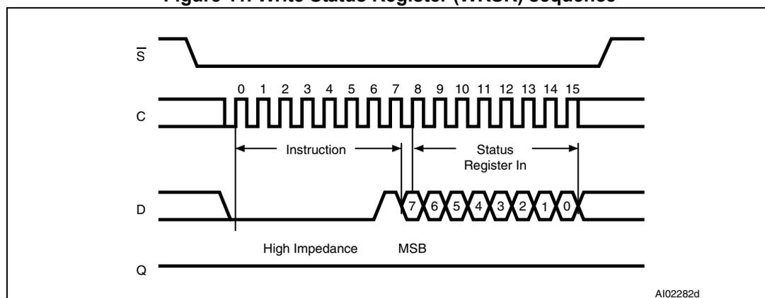
Driving the Chip Select ( $\bar{S}$ ) signal high at a byte boundary of the input data triggers the self-timed Write cycle that takes  $t_{WV}$  to complete (as specified in AC tables under [Section 9: DC and AC parameters](#)).
