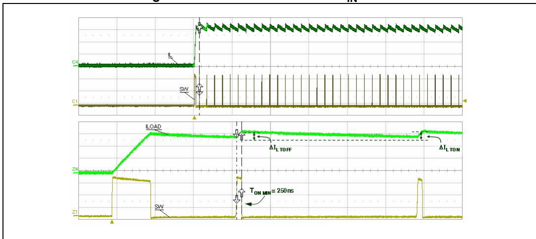
Figure 21. Short-circuit current V_{IN} = 36\text{ V}
