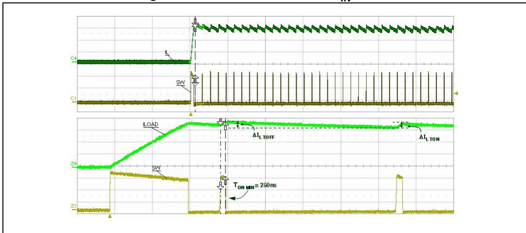
Figure 20. Short-circuit current V_{IN} = 24\text{ V}
