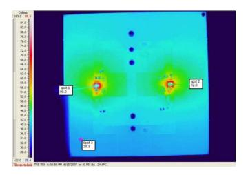
Figure 6. Temperature Rise at 1.7W Dissipation
