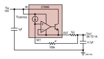
Low Dropout Voltage LED Driver
