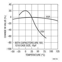
Figure 3. Ceramic Capacitor Temperature Characteristics
