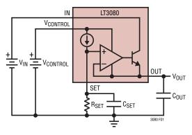
Figure 1. Basic Adjustable Regulator
