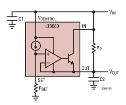
Figure 9. Reducing Power Dissipation Using a Parallel Resistor
