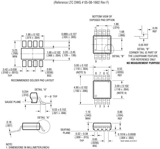
**MS8E** Package 8-Lead Plastic MSOP, Exposed Die Pad
