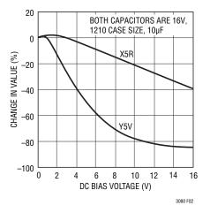
Figure 2. Ceramic Capacitor DC Bias Characteristics
