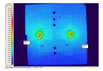
Figure 5. Temperature Rise at 700mW Dissipation
