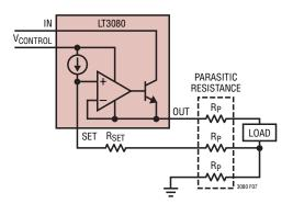
Figure 7. Connections for Best Load Regulation
