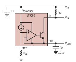
Figure 8. Reducing Power Dissipation Using a Series Resistor
