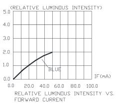
The above data are collected from statistical figures that do not necessarily correspond to the actual parameters of each single LED. Hence, these data will be changed without further notice.
