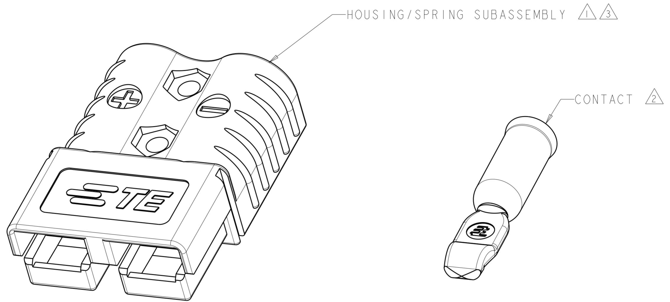
⚠ HOUSING MATERIAL: POLYCARBONATE UL 94 V-0
