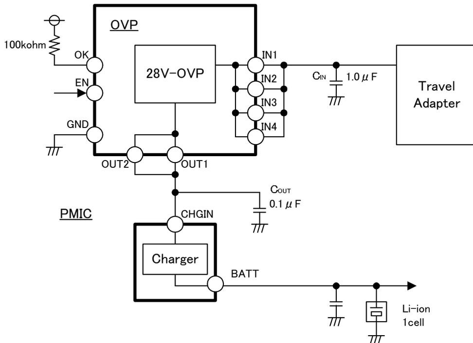
Fig. 17 Application Circuit
