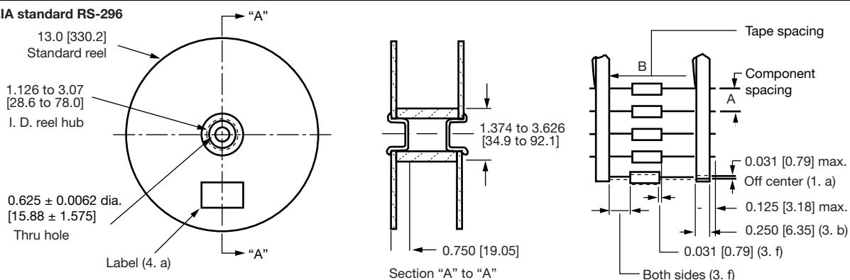
**STANDARD PACKAGING QUANTITY AND DIMENSIONS** in inches [millimeters]
