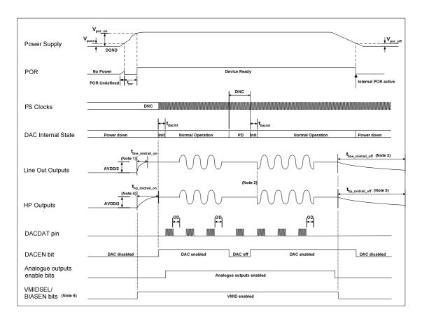
Figure 35 DAC Power Up and Down Sequence (not to scale)
