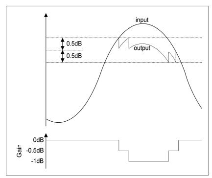
Figure 19 DAC Digital Limiter Operation
