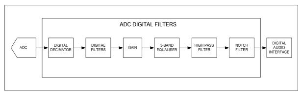
Figure 10 ADC Digital Filter Path
