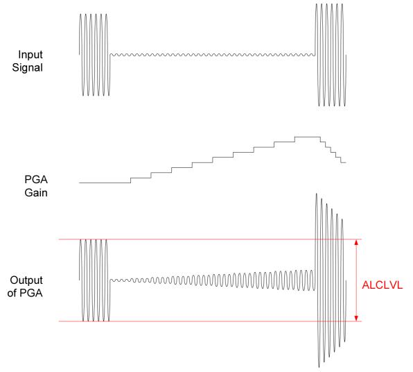
Figure 16 ALC Operation Above Noise Gate Threshold
