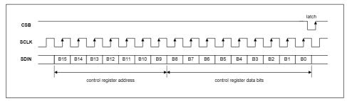
Figure 32 3-Wire Serial Control Interface
