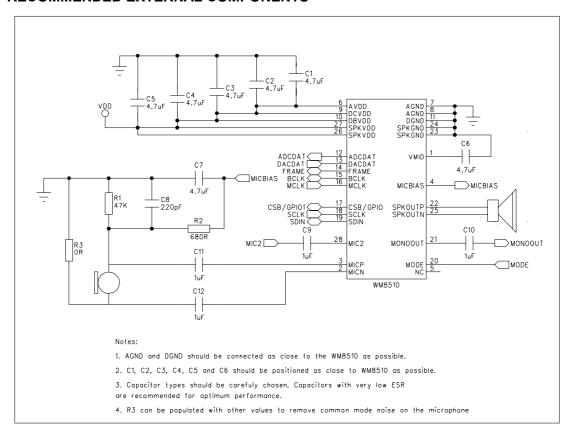
Figure 50 Recommended External Components
