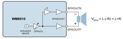
Figure 22 Speaker Output Connection
