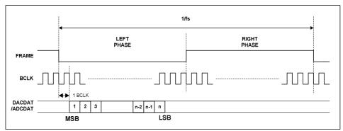
Figure 27 I<sup>2</sup>S Audio Interface (assuming n-bit word length)
