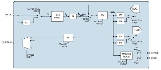
Figure 31 PLL and Clock Select Circuit
