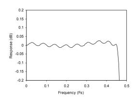
Figure 38 ADC Digital Filter Frequency Response
