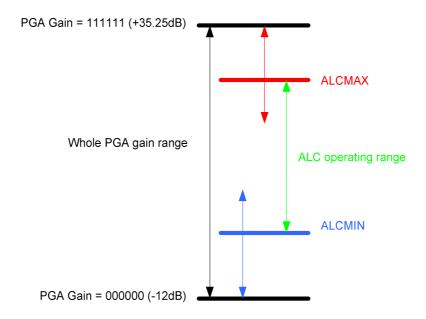
Figure 13 ALC Min/Max Gain
