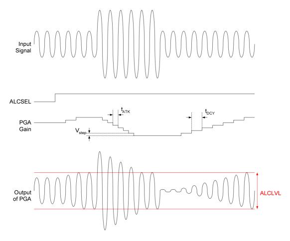
Figure 11 ALC Normal Mode Operation
