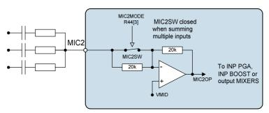
Figure 7 MIC2 Input Circuit
