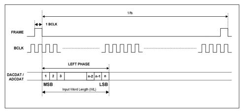
Figure 28 DSP/PCM Mode Audio Interface (mode A)
