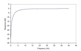
Figure 46 ADC Highpass Filter Response, HPFAPP=0
