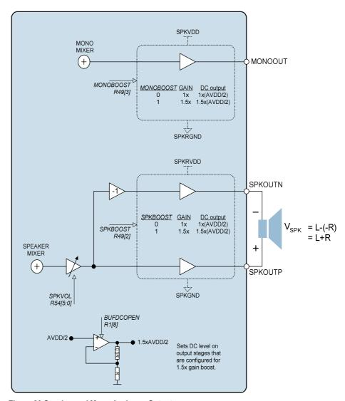
Figure 20 Speaker and Mono Analogue Outputs
