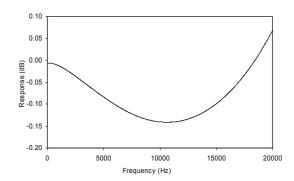
Figure 42 De-emphasis Frequency Response (44.1kHz)
