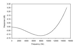
Figure 40 De-emphasis Frequency Response (32kHz)
