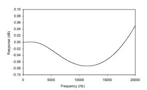
Figure 44 De-emphasis Frequency Response (48kHz)
