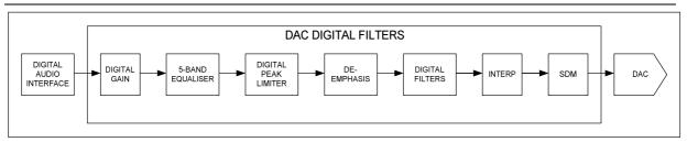
Figure 18 DAC Digital Filter Path
