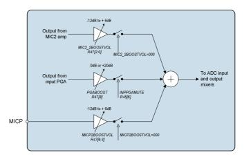
Figure 8 Input Boost Stage
