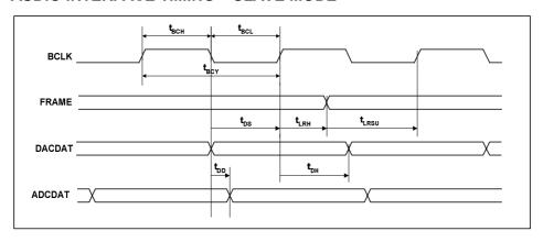
Figure 3 Digital Audio Data Timing - Slave Mode
