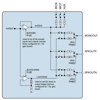
Figure 21 Unused Input/Output Pin Tie-off Buffers
