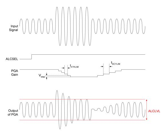
Figure 12 ALC Limiter Mode Operation
