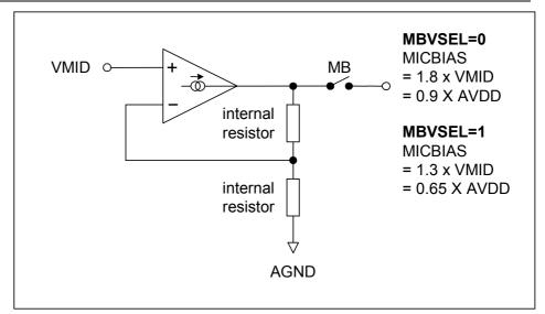
Figure 9 Microphone Bias Schematic
