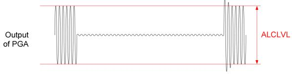
Figure 17 Noise Gate Operation
