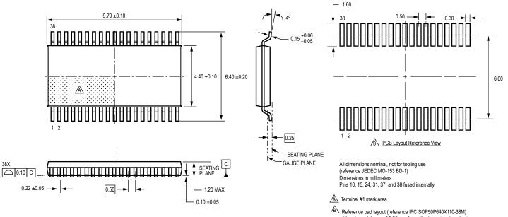
All pads a minimum of 0.20 mm from all adjacent pads; adjust as necessary to meet application process requirements and PCB layout tolerances
