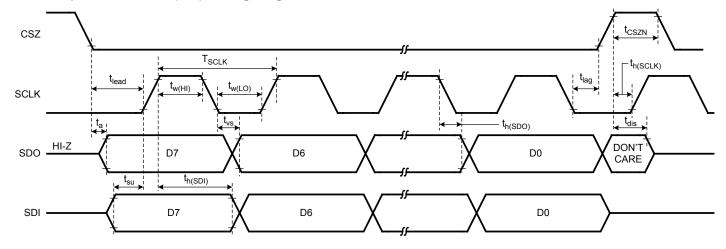
Serial Peripheral Interface (SPI) Timing Diagram
