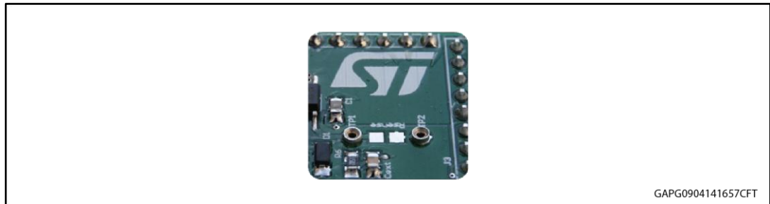
Figure 4: Mounting through-hole sense resistor
