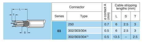
**Note:** the tolerances on these dimensions are: L:  $\pm$  0.5 mm; S:  $\pm$  0.5 mm; T:  $\pm$  0.2 mm. <sup>1)</sup> for FVG model with cable crimping.
