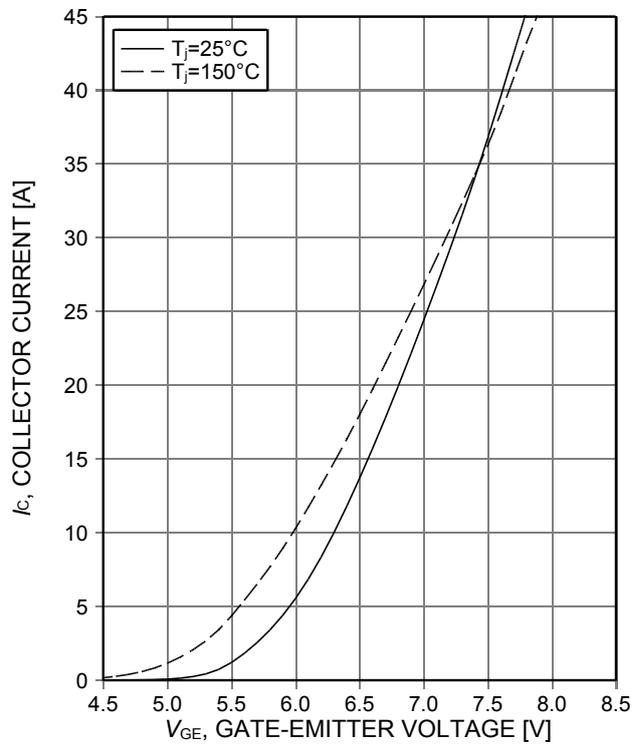
Figure 6. Typical transfer characteristic ( $V_{CE}=20\text{V}$ )
