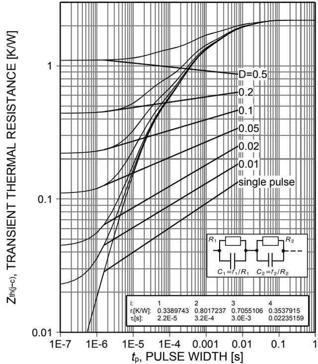
Figure 18. IGBT transient thermal resistance ( $D=t_p/T$ )
