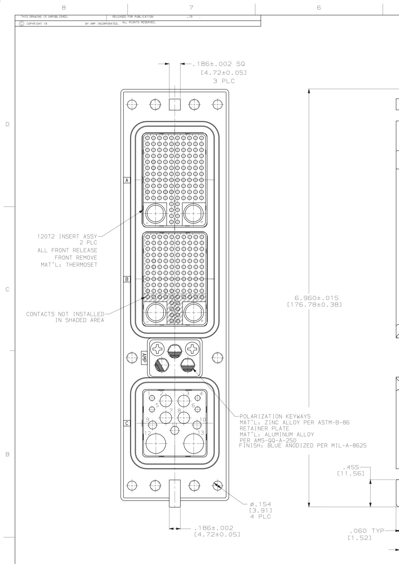
1. CONNECTOR DIMENSIONS ARE PER ARINC 600 SPECIFICATION.
