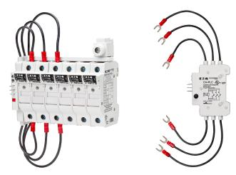
The Bussmann series resettable PLC fuse monitor permits easy integration with a Programmable Logic Controller (PLC) or other monitoring and control equipment. Signals up to three-phases. Includes 0.11" (2.8 mm) quick-connects for power, signal and ground connections.
