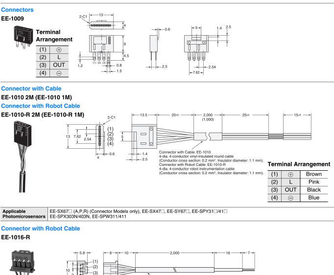
2.8-dia. 4-conductor robot instrumentation cable (Conductor cross section: 0.15 mm², Insulator diameter: 0.8 mm); Standard length: 2 m
