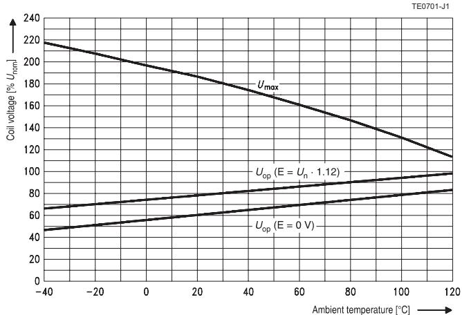
Does not take into account the temperature rise due to the contact current E=pre-energization..
