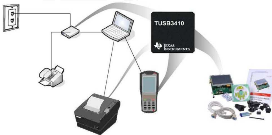
Figure 6-1. Typical Example for TUSB3410 as USB to UART Bridge
