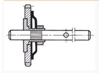
This device is situated inside the gearbox and is particularly recommended when gearbox protection is required in the event of accidental overloading. In this system, the final gear is connected to the gearbox output shaft by means of a friction assembly. In some cases, this device can be used for time adjustment or zero reset on timers.
