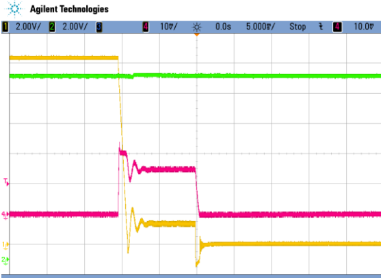
Figure 9 - Turn-On AC Line 230 VAC, full load (5 ms/div) CH2: VSB (2 V/div)
