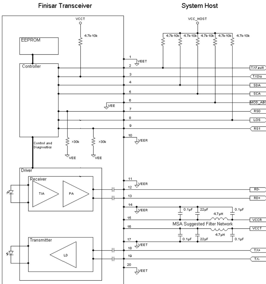
**Figure 6-Host-Module Interface**
