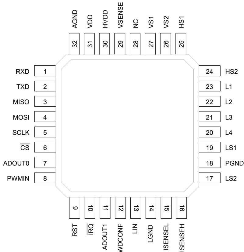
Figure 3. 33912 pin connections
