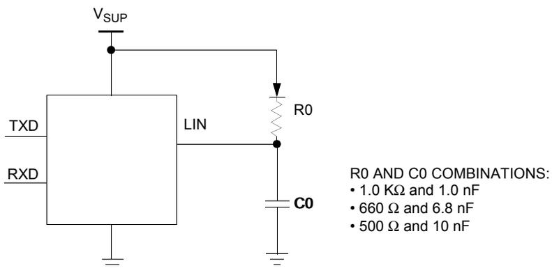
**Figure 29. Test circuit for LIN timing measurements**
