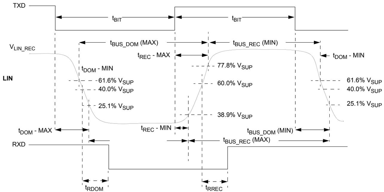
Figure 31. LIN timing measurements for slow slew rate
