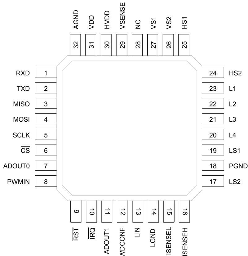
**Figure 26. 33912 pin connections**
