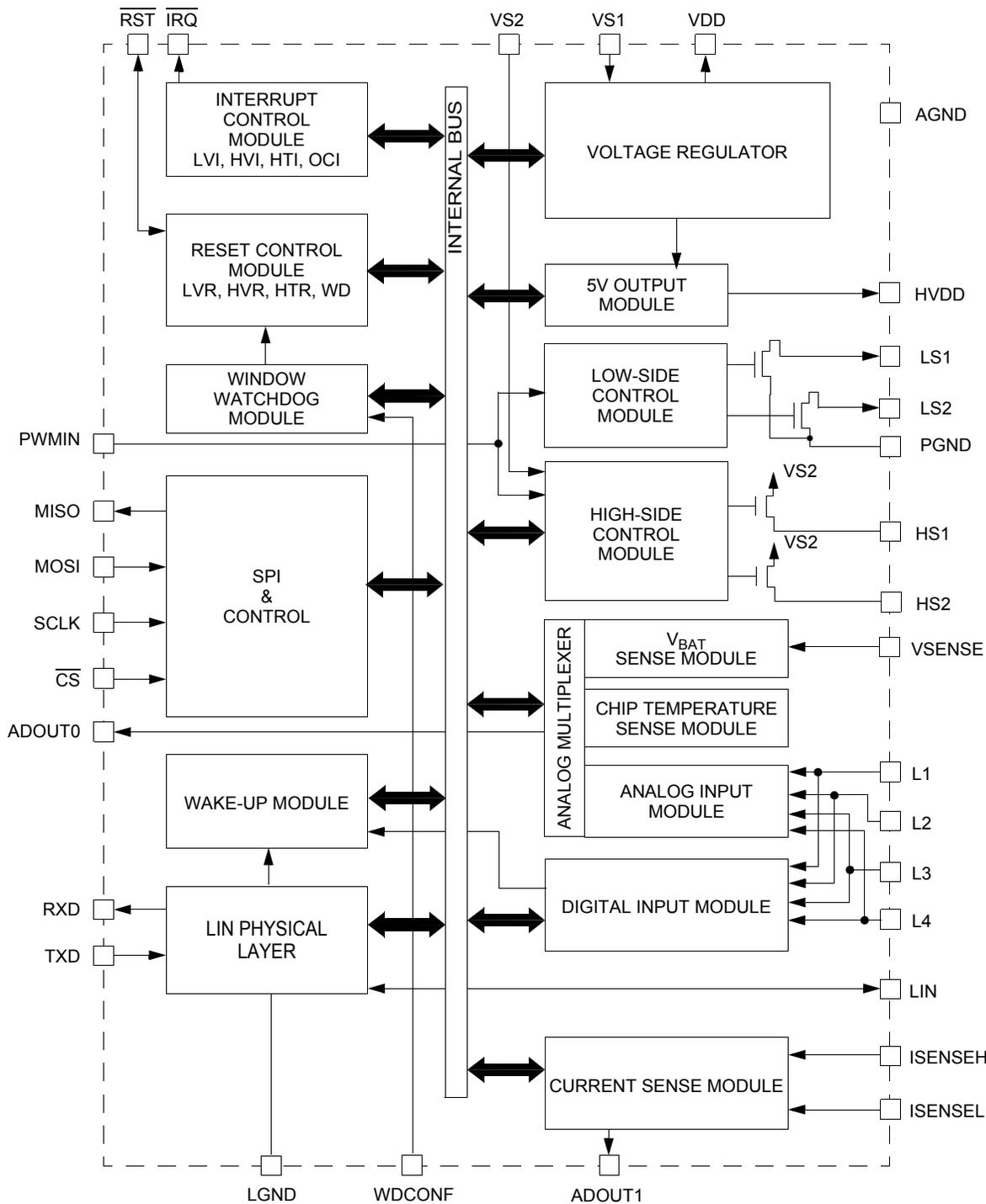
Figure 25. 33912 simplified internal block diagram
