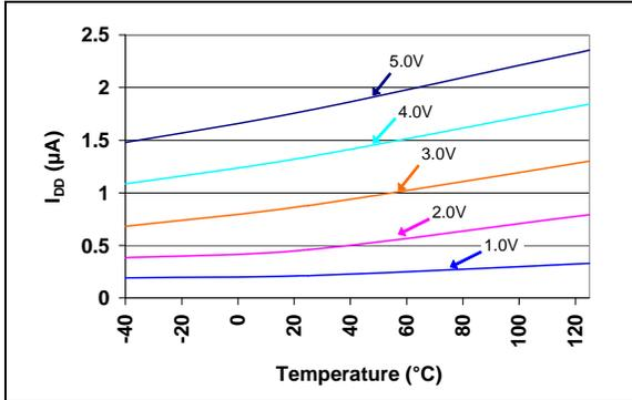
**FIGURE 2-1:**  $I_{DD}$  vs. Temperature (Reset Power-up Timer Inactive)
