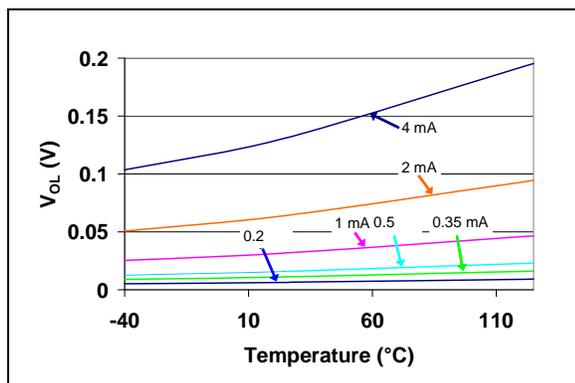
**FIGURE 2-21:**  $V_{OL}$  vs. Temperature
