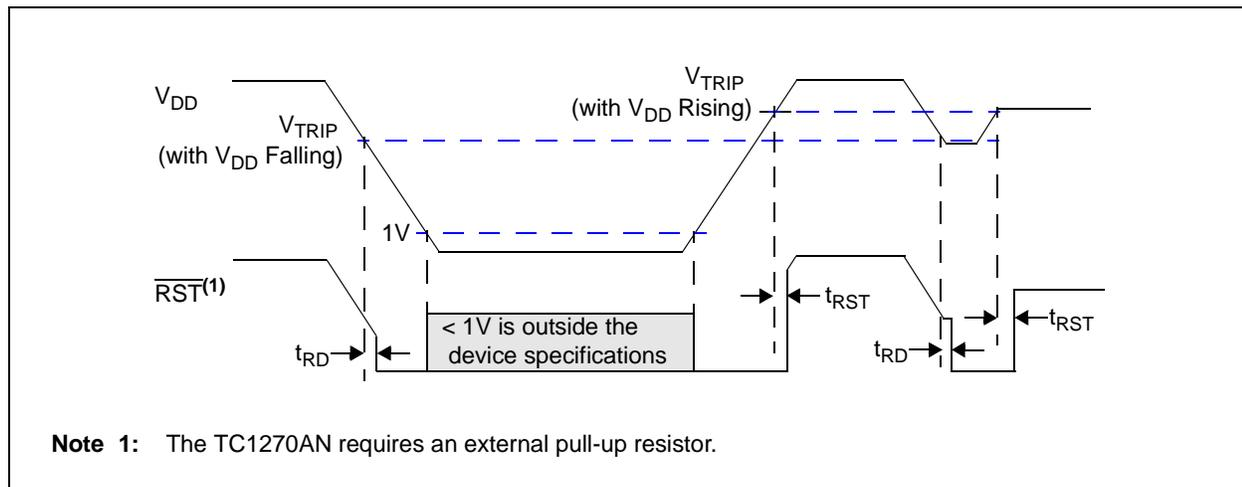
**FIGURE 4-8:**  $\overline{RST}$  Operation as determined by the  $V_{TRIP}$
