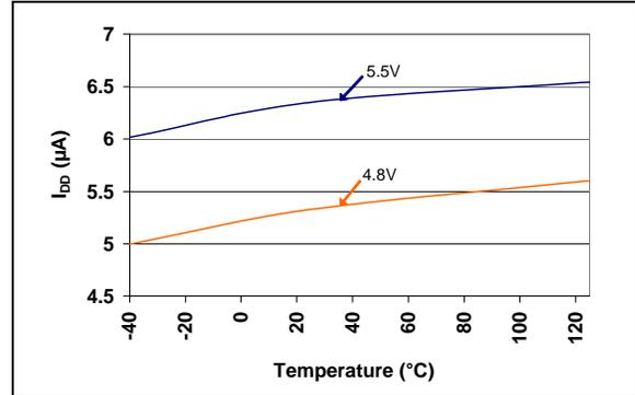
**FIGURE 2-4:**  $I_{DD}$  vs. Temperature (Reset Power-up Timer Active)
