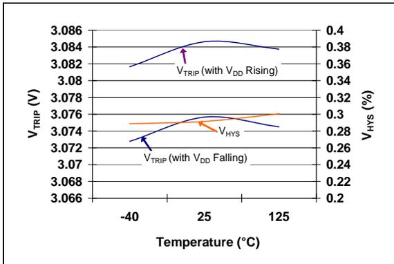
**FIGURE 2-14:**  $V_{TRIP}$  and  $V_{HYS}$  vs. Temperature
