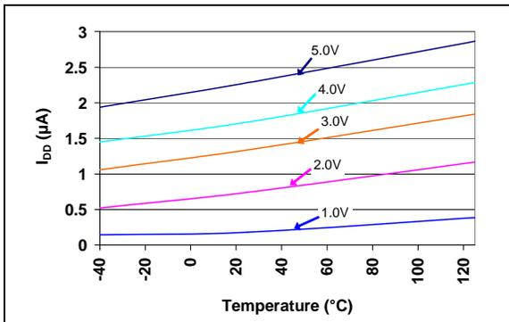
**FIGURE 2-3:**  $I_{DD}$  vs. Temperature (Reset Power-up Timer Inactive)
