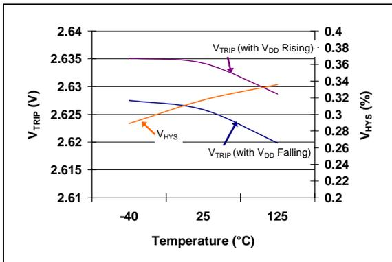
**FIGURE 2-15:**  $V_{TRIP}$  and  $V_{HYST}$  vs. Temperature
