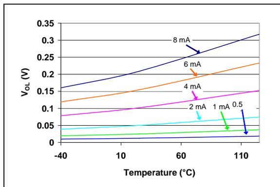
**FIGURE 2-20:**  $V_{OL}$  vs. Temperature
