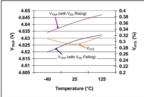
**FIGURE 2-13:**  $V_{TRIP}$  and  $V_{HYS}$  vs. Temperature
