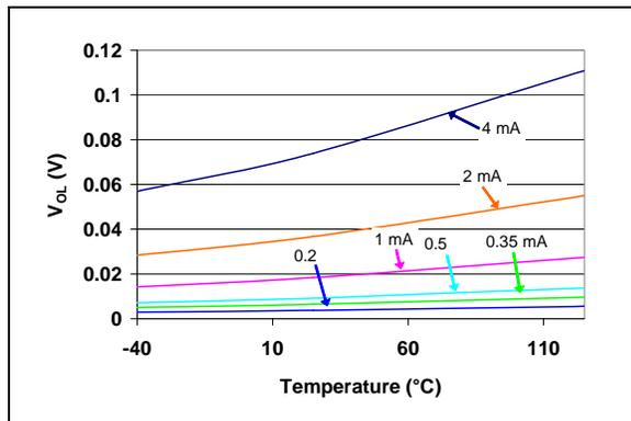
**FIGURE 2-19:**  $V_{OL}$  vs. Temperature
