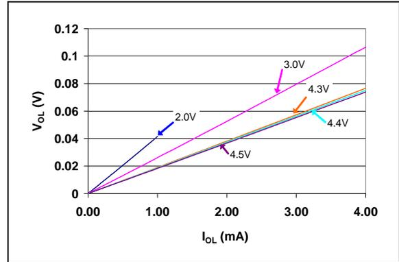
**FIGURE 2-16:**  $V_{OL}$  vs.  $I_{OL}$
