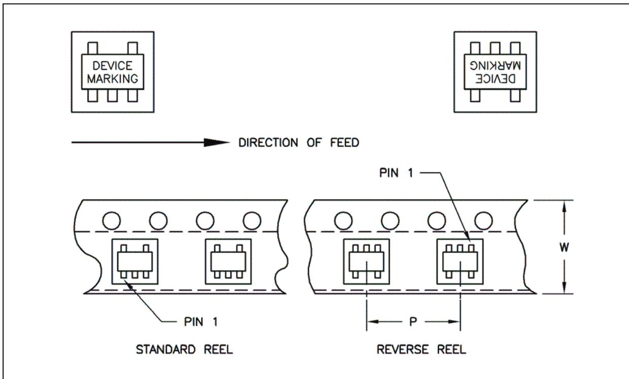
**FIGURE 9-3: 4-LEAD SOT-143 DEVICE TAPE AND REEL SPECIFICATIONS**
