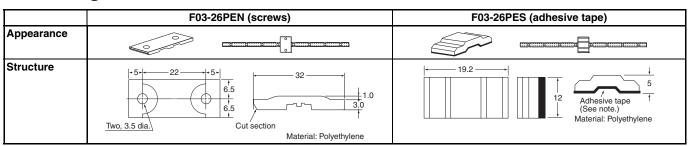
Note: The shape of the adhesive tape shown above is for securing the F03-16PE.
