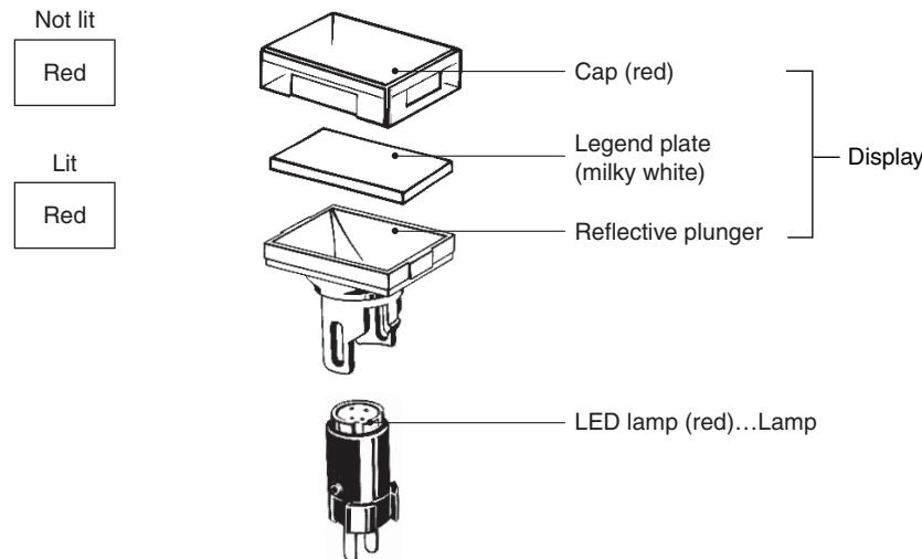
“Colored illumination” describes LED models for which the screen color is white when the LED is not lit and changes to the color of the LED lamp when the LED is lit.
