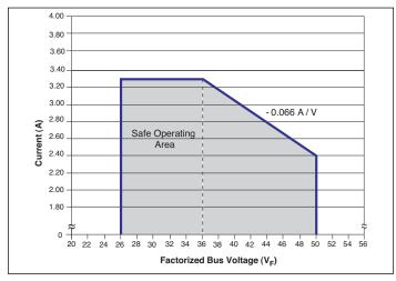
Figure 19 — MP028F036M12AL rating based on Factorized Bus voltage
