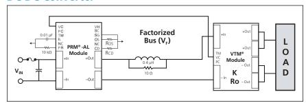
The MP028F036M12AL is used with any 036 input series VTM™ module to provide a regulated and isolated output.
