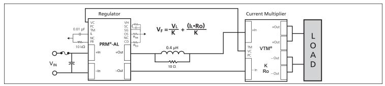
**Figure 18** — Adaptive Loop compensation with output voltage trimming and soft start using the SC port.
