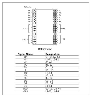
Figure 17 — PRM pin configuration
