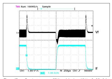
**Figure 12** — Transient response; PRM module alone 16 V<sub>IN</sub>, 0–3.3–0 A, no load capacitance, local loop
