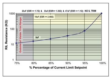
**Figure 20** —  $R_{lL}$  vs percentage of current limit. Shaded areas shown minimum valid  $R_{ll}$  as a function of load capacitance and ESR.
