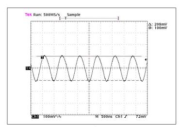
**Figure 16** — Output ripple 36 V<sub>OUT</sub>, full load 10 μF bypass capacitance
