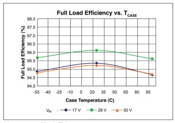
Figure 10 — Full load efficiency vs T<sub>CASE</sub>
