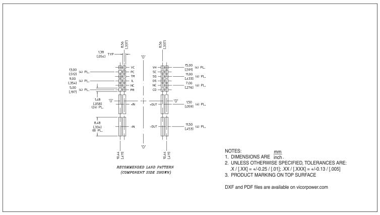
Figure 22 — PRM™ module J-Lead PCB land layout information
