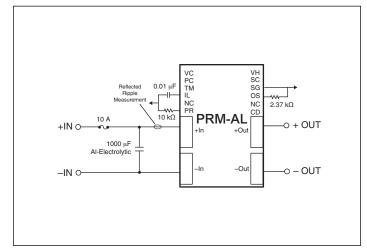
**Figure 5** — Input filter capacitor recommendation
