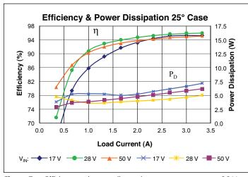
**Figure 7** — Efficiency and power dissapation vs. output current at 36  $V_{OUT}$ , 25 °C  $T_{CASE}$
