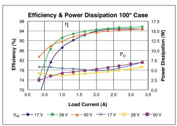
**Figure 8** — Efficiency and power dissapation vs. output current at 36  $V_{OUT}$ , 100 °C  $T_{CASF}$
