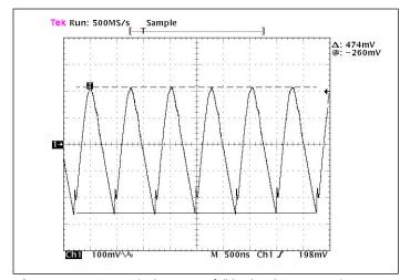
**Figure 15** — Output ripple 36 V<sub>OUT</sub>, full load no bypass capacitance
