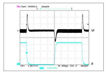
**Figure 11** — Transient response; PRM module alone 28 V<sub>IN</sub>, 0–3.3–0 A, no load capacitance, local loop
