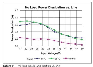
**rigure 9** — No load power, unit enabled vs. line
