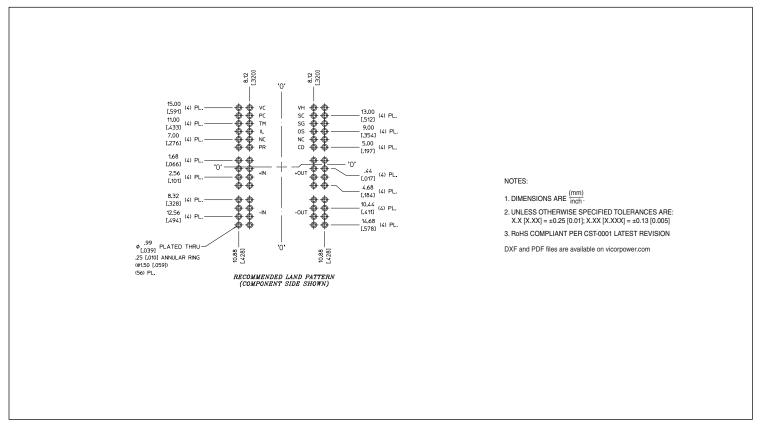
**Figure 24** — PRM™ moduel through-hole PCB layout information
