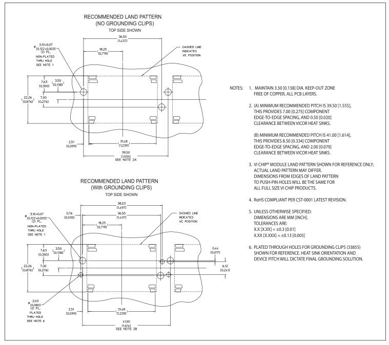
Figure 25 — Recommended heat sink push pin location
