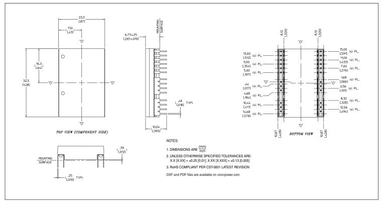
Figure 23 — PRM™ module through-hole mechanical outline
