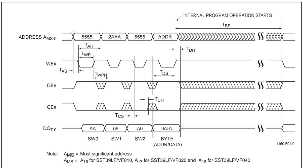
Figure 5: WE# Controlled Program Cycle Timing Diagram
