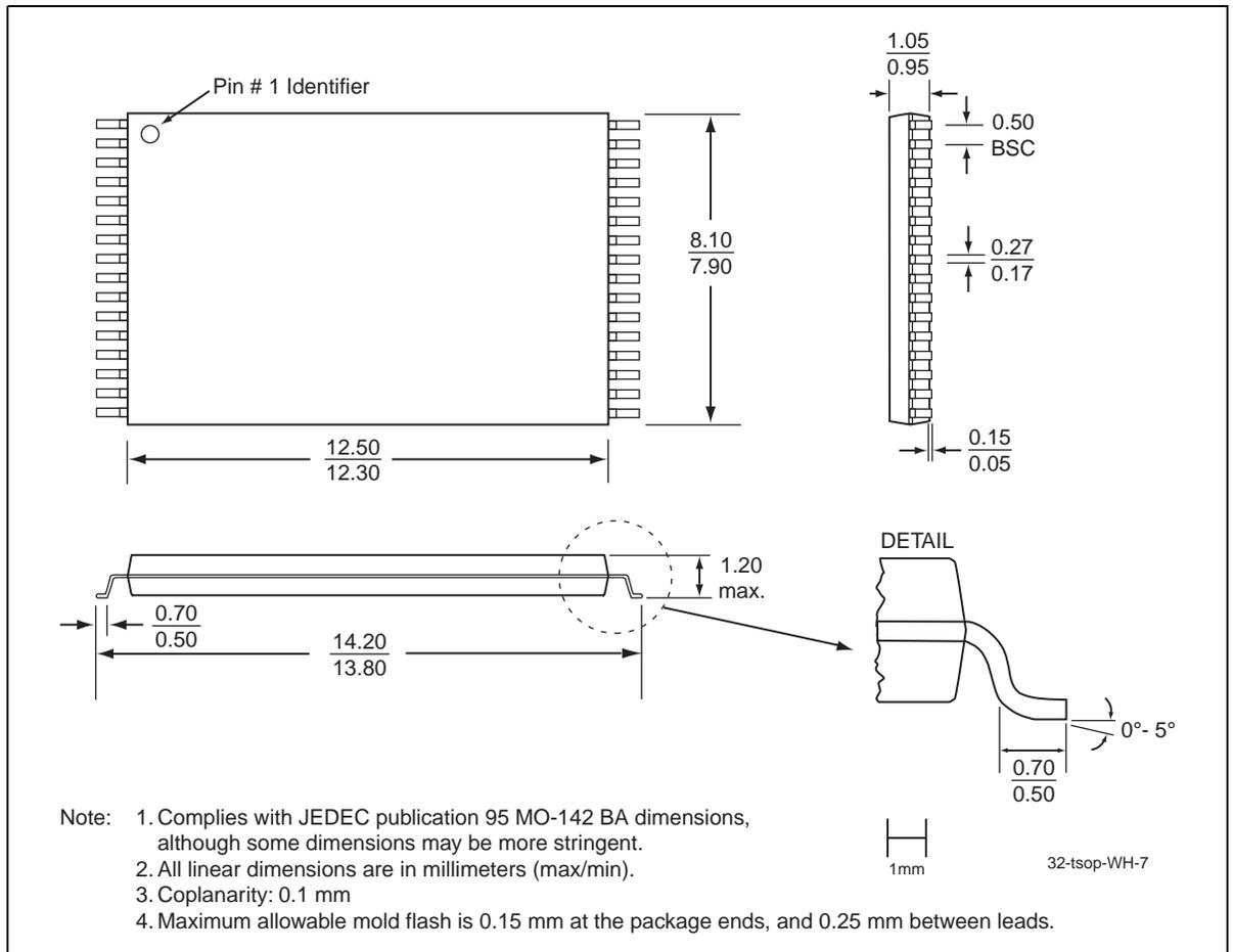
**Figure 20:** 32-lead Thin Small Outline Package (TSOP) 8mm x 14mm
