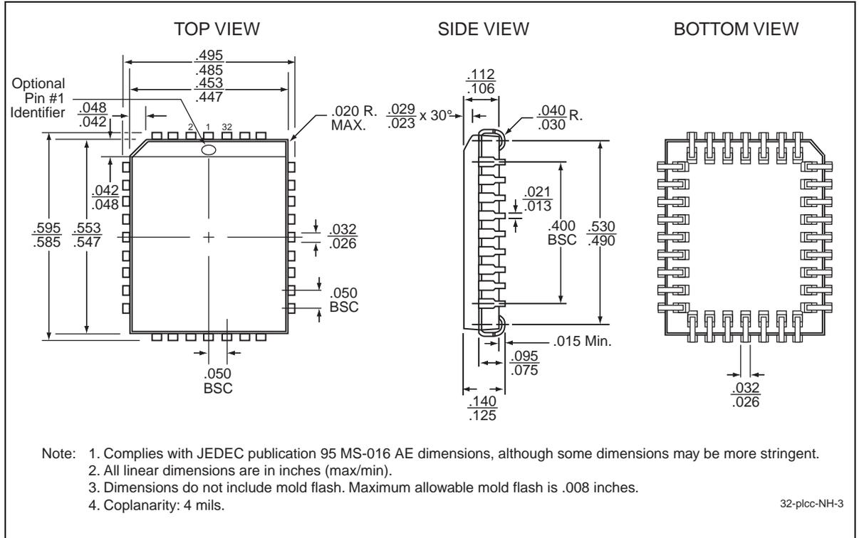
**Figure 19:**32-lead Plastic Lead Chip Carrier (PLCC)
