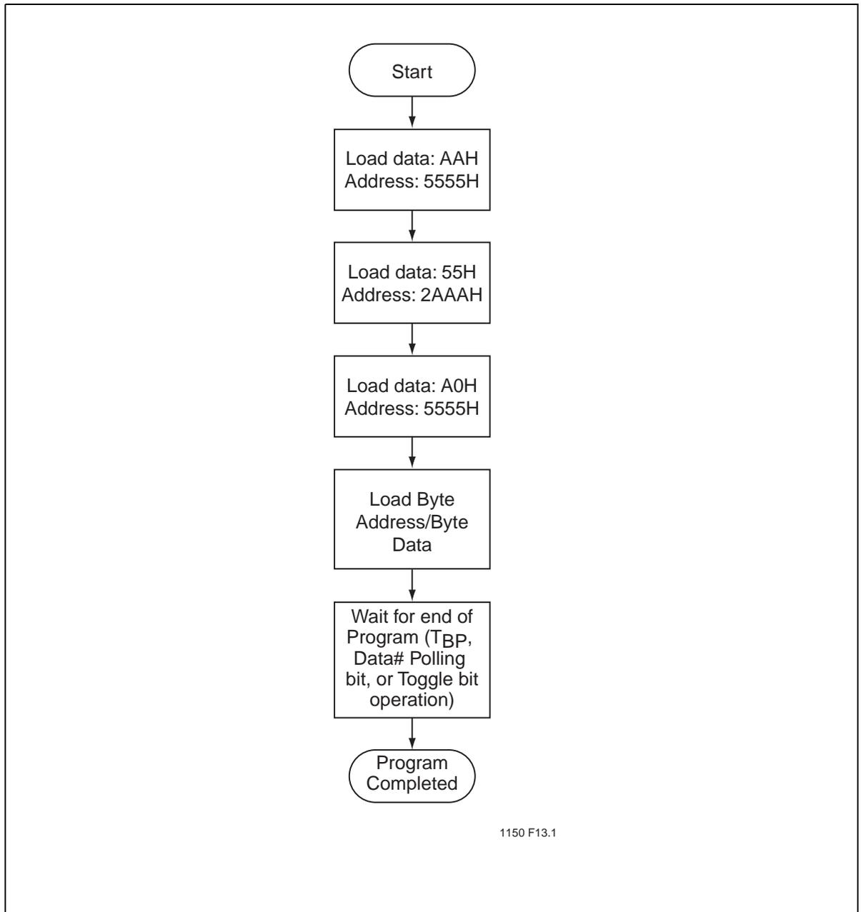
**Figure 15:**Byte-Program Algorithm
