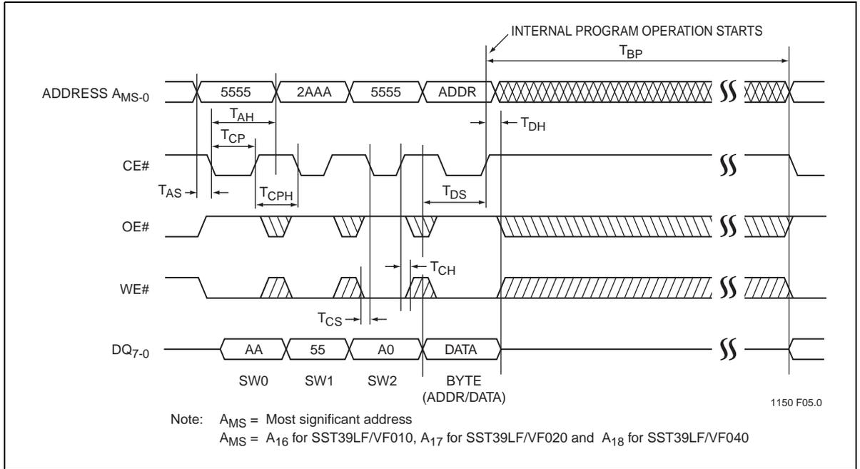
**Figure 6:** CE# Controlled Program Cycle Timing Diagram
