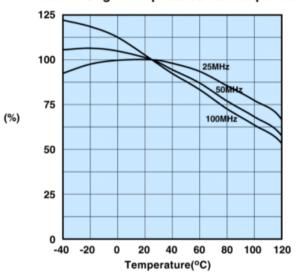
Measured on a 2643000301 using the HP4291A.
