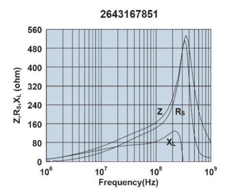
Impedance, reactance, and resistance vs. frequency.
