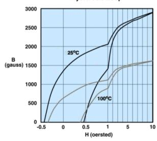
Measured on a 17/10/6mm toroid at 10kHz.
