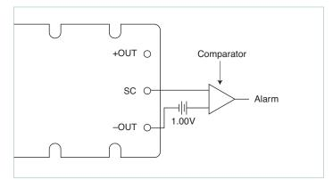
Figure 7 — Secondary-side on-state indicator
