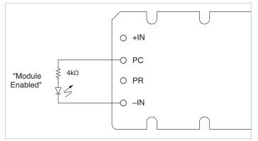
Figure 4 — LED on-state indicator
