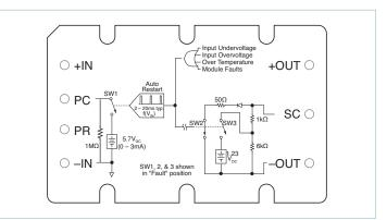
Figure 3 — PC/SC module alarm logic
