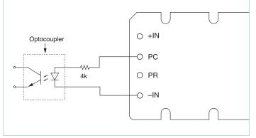
Figure 6 — Isolated on-state indicator
