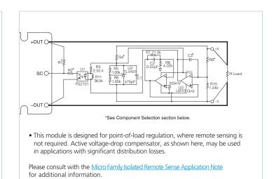
Figure 12 — Voltage-drop compensation
