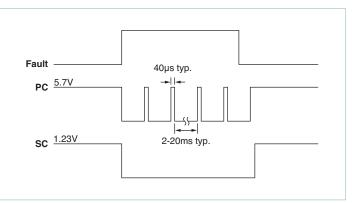
Figure 5 — PC/SC module alarm timing
