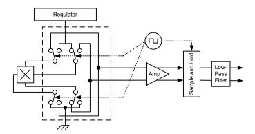
Figure 2: Chopper Stabilization Circuit (Dynamic Quadrature Offset Cancellation)
