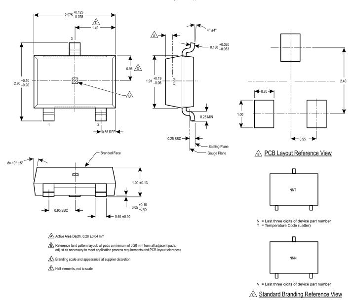
Figure 5: Package LH, 3-Pin SOT23W
