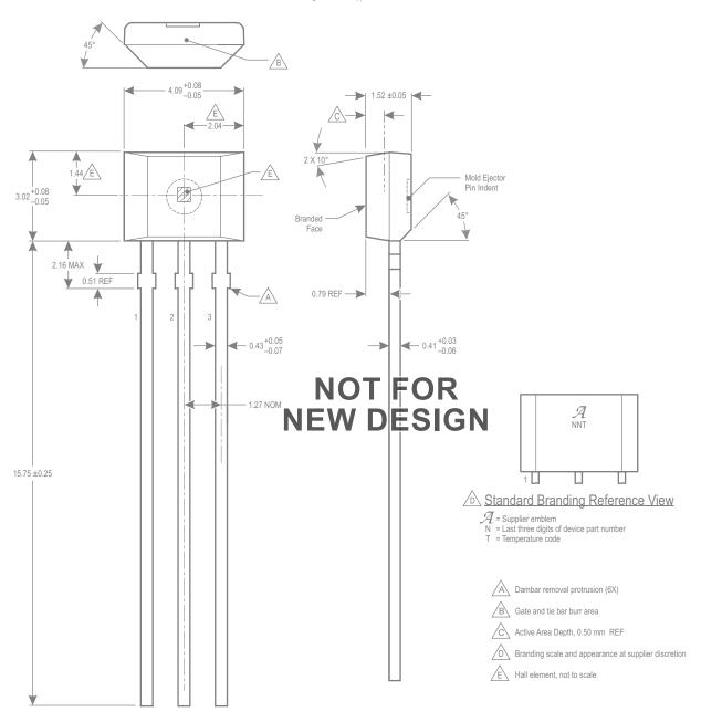
Figure 7: Package UA, 3-Pin SIP, Chopper Style (A3290)
