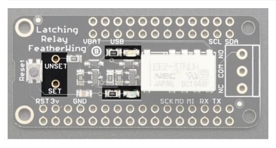
The latching relay uses two pins for control. There is no way to know which 'orientation' the relay is when the Feather turns on, because the relay will latch in the last position it was set to.
