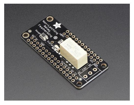
Both FeatherWings use the same family of relay. You can switch up to 2A of resistive current at 30VDC or ~40VAC or lower. At 110VDC you can switch up to 0.3A, at 120VAC up to 0.5A, and at 250VAC you can switch up to 0.6A. Check the datasheet for the relay for the exact switching capacity, and of course, for reactive/inductive loads you will need to derate. This isn't a relay you can use to turn on and off your washer/dryer, stick to 60W or less.
