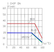
MAXIMUM FORWARD DC CURRENT VS, AMBIENT TEMPERATURE.
