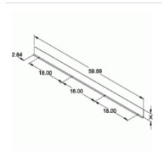
• Divides wireway into two or more compartments. Barriers are fastened to wireway sections with screws.
